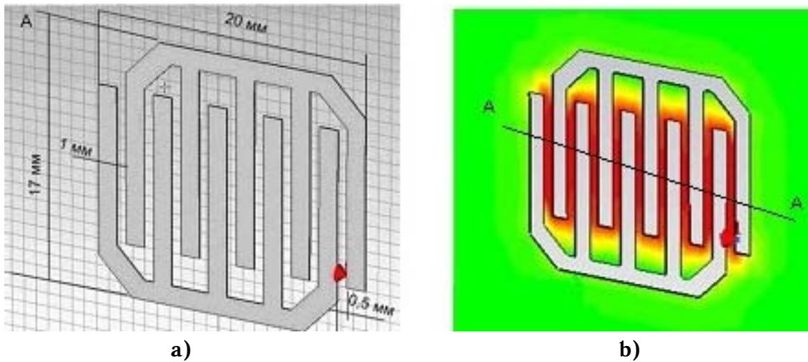
Fig. 2. Radio-frequency antenna-sensor: a) Overview of the antenna geometry; b) Quasi-static field (near-field zone) at the antenna aperture
