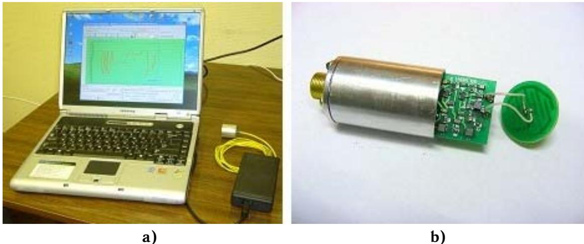
Fig. 1. Diagnostic radio-frequency near-field probing equipment: a) general overview of the equipment in full assembly; b) overview of the antenna-sensor with circuit board of the RF generator
