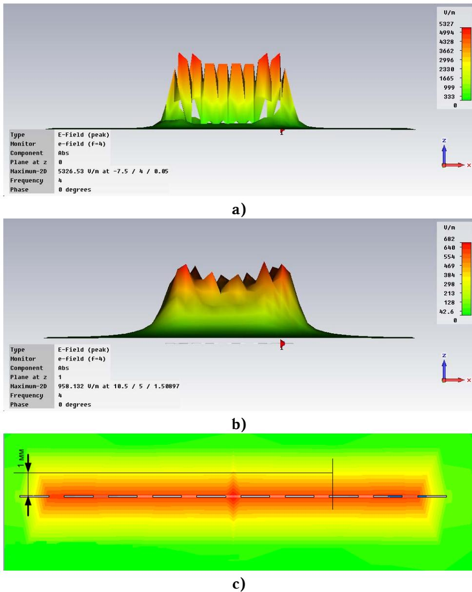
Fig. 3. Quasi-static electric field distribution at the antenna aperture (near-field zone): a) field distribution at A-A cross-section (Figure 2-b). b) Distribution of the same field (a) 1mm away from antenna's aperture. Note that field amplitude is decreased by approx. 10 times. c) field distribution at 90 degrees
