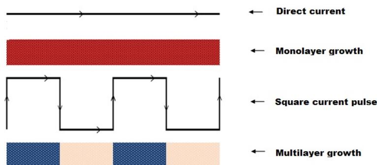
FIG. 1. Power pattern used for the deposition of monolayer (Direct current) and multilayer (square current pulse) coatings
