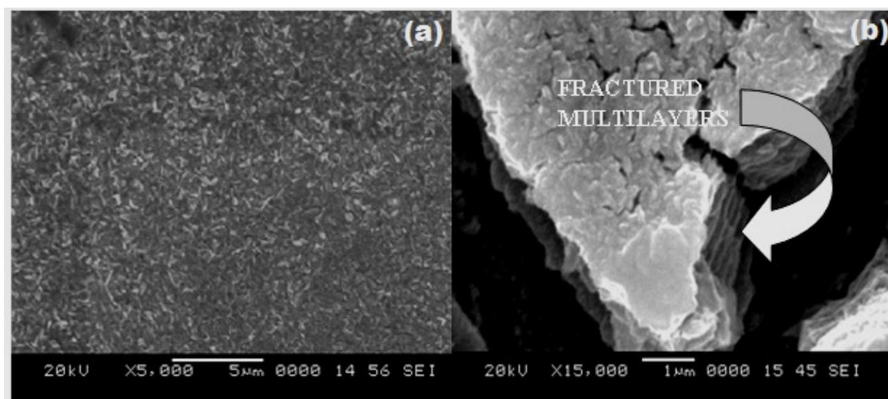
FIG. 4. SEM images of NMC  $(\text{Zn-Ni})_{2.0/4.0/10}$  coatings electrofabricated from optimized bath: (a) surface structure and (b) cross-sectional view after bend test
