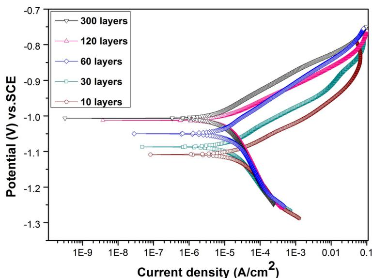
FIG. 2. Potentiodynamic polarization behaviors of NMC (Zn-Ni) coatings having different number of layers, deposited from optimized bath at 303 K
