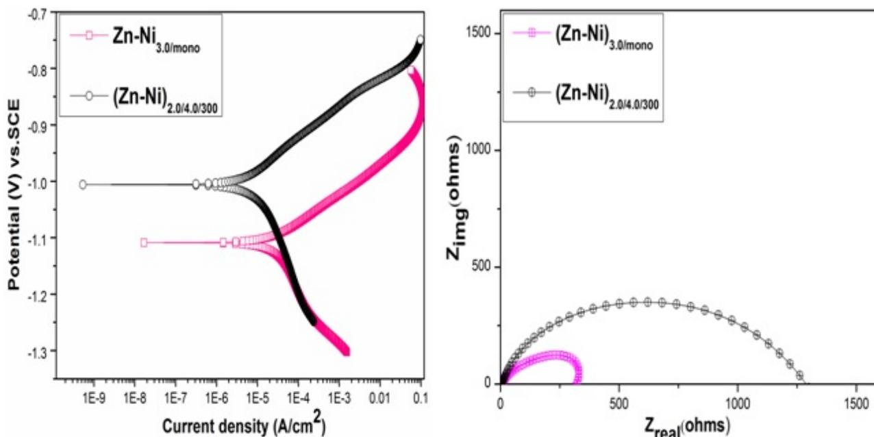
FIG. 3. Comparison of corrosion behaviors of monolayer and multilayer coatings of (Zn-Ni) alloy: a) Potentiodynamic polarization behaviors and b) Nyquist response under same frequency limit
