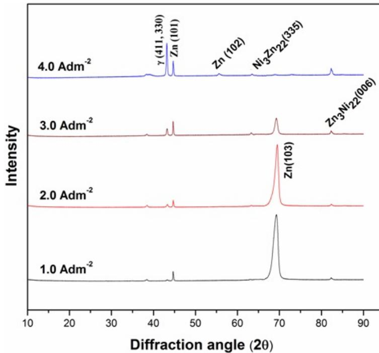
FIG. 5. XRD patterns of Zn-Ni alloy coatings at different c.d.s.
