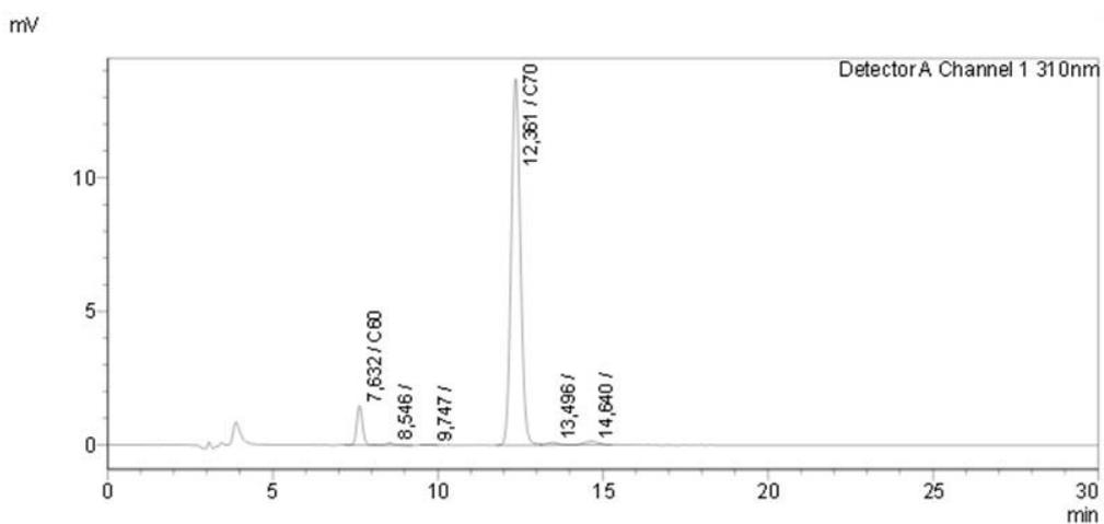
FIG. 4. Liquid — phase chromatograms of mixture  $C_{60} + C_{70}$
