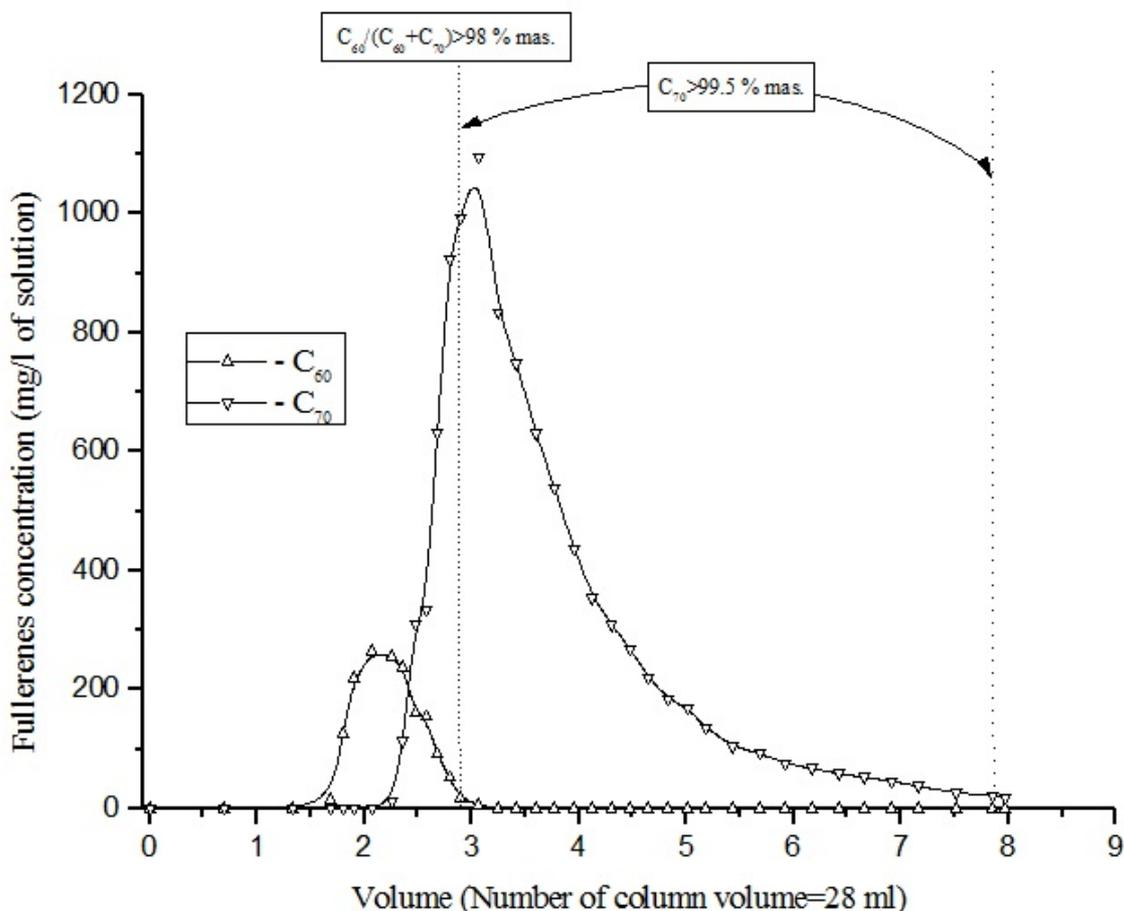
FIG. 10. Chromatographic separation of light fullerenes  $C_{60}$  and  $C_{70}$  with the help of the sorbent Bayer Multiwall Carbon Nanotubes from toluene solutions
