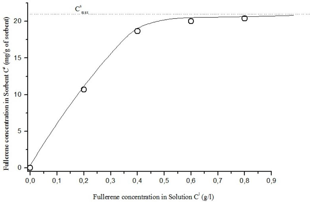
FIG. 6. Sorption isotherms in the  $C_{60}$  fullerene – Bayer MWCNTs – toluene system in normal coordinates
