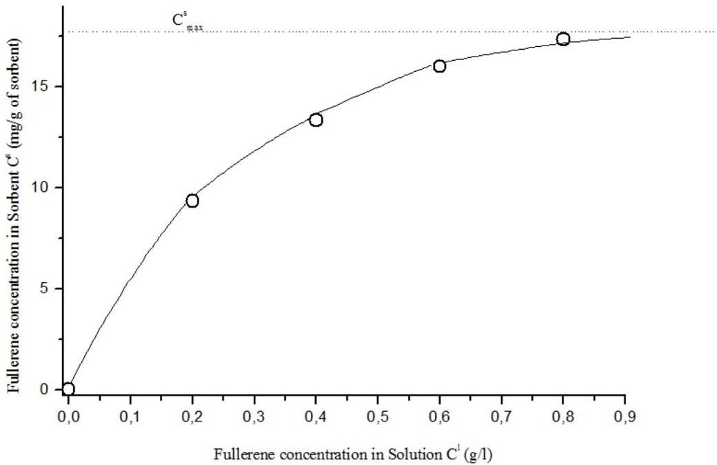
FIG. 7. Sorption isotherms in the  $C_{70}$  fullerene – Bayer MWCNTs – toluene system in normal coordinates
