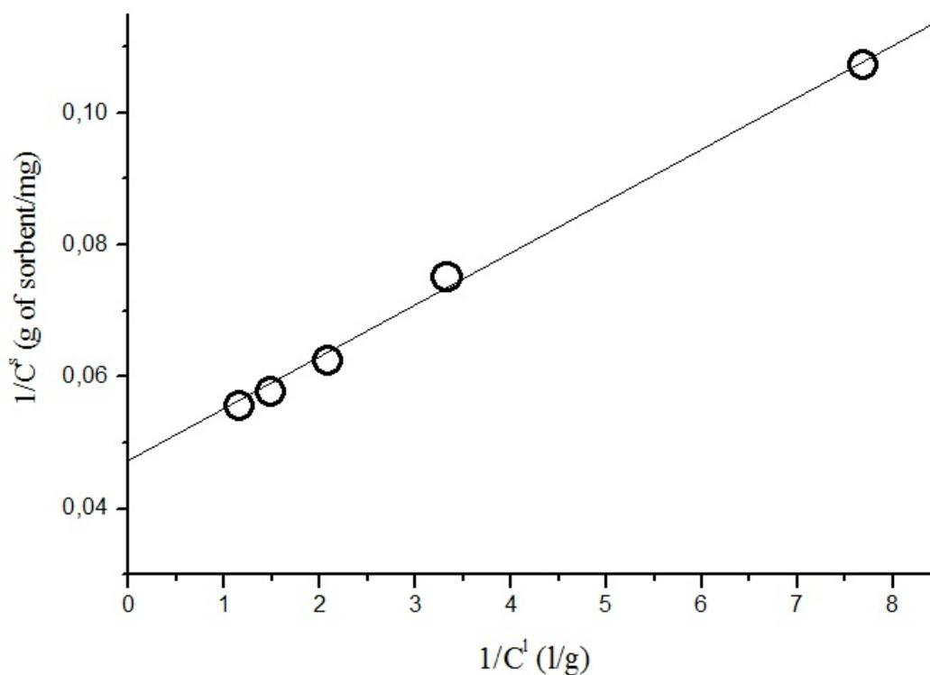
FIG. 9. Sorption isotherms in the  $C_{70}$  fullerene – Bayer MWCNTs – toluene system in Langmuir coordinates
