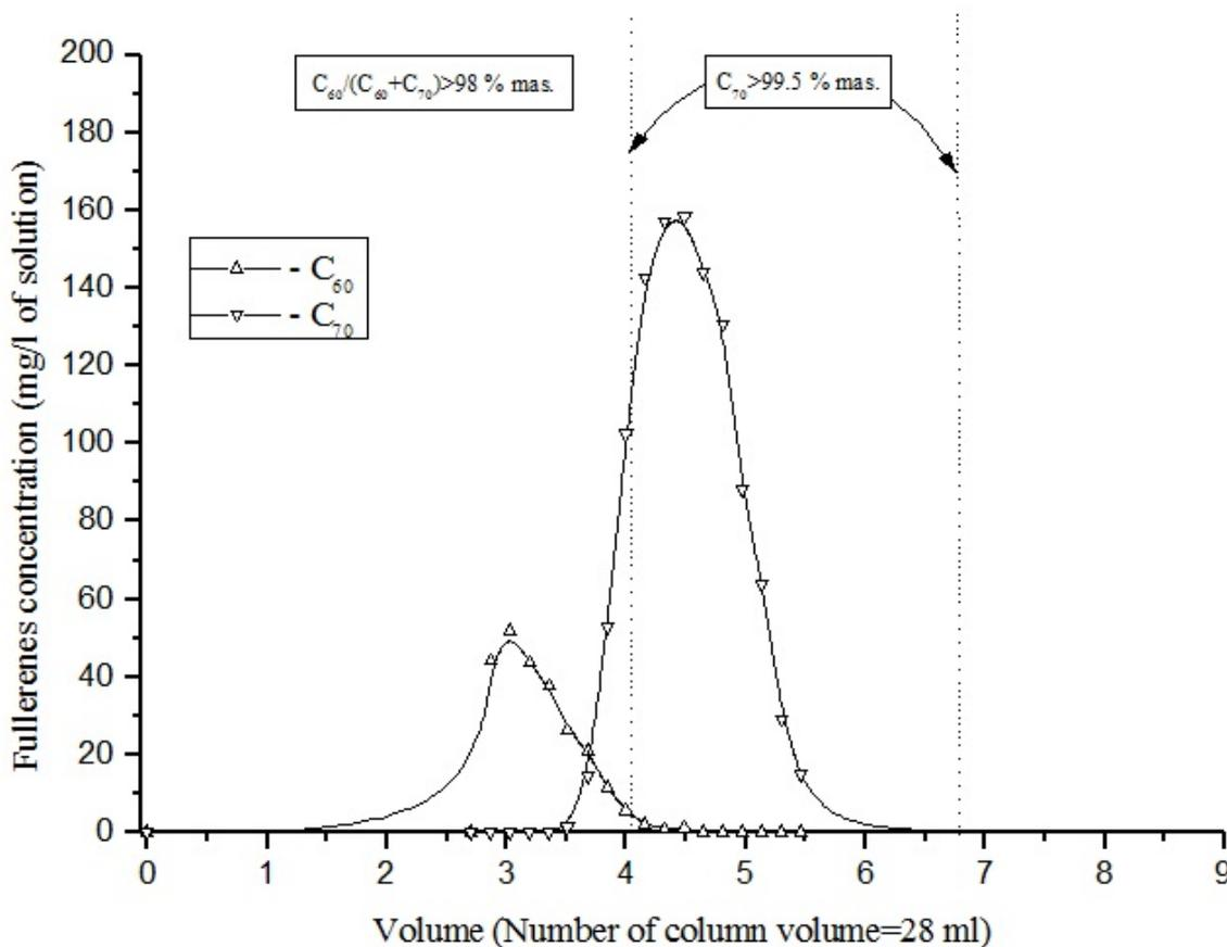
FIG. 11. Chromatographic separation of light fullerenes  $C_{60}$  and  $C_{70}$  with the help of the mixed sorbent Bayer MWCNTs/granules of fluorine plastic from toluene solutions
