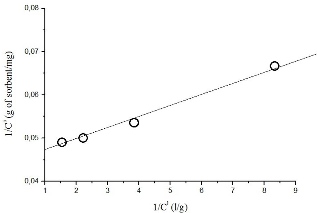
FIG. 8. Sorption isotherms in the  $C_{60}$  fullerene – Bayer MWCNTs – toluene system in Langmuir coordinates
