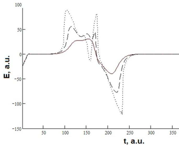
FIG. 2. Time dependence of the pulse form for different cases of pulse amplitude value: a) solid line –  $Q = 2$ ; b) dotted line –  $Q = 3$ ; c) dashed line –  $Q = 5$ . Time and electric field a.u. as in Fig. 1
