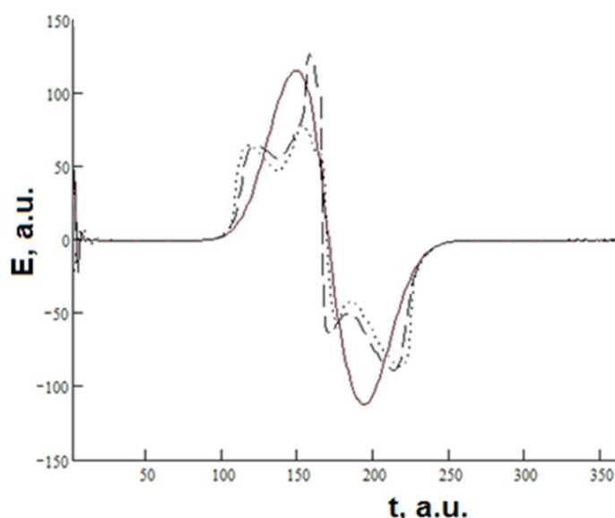
FIG. 3. Time dependence of the electric field on time taking into account the nonlinear polarization of the medium: a) solid line –  $\beta = 0.03$ ; b) dotted line –  $\beta = 0.4$ ; c) dashed line –  $\beta = 0.6$  the dispersion is almost zero,  $\alpha = 0.01$ . Time and electric field a.u. as in Fig.1
