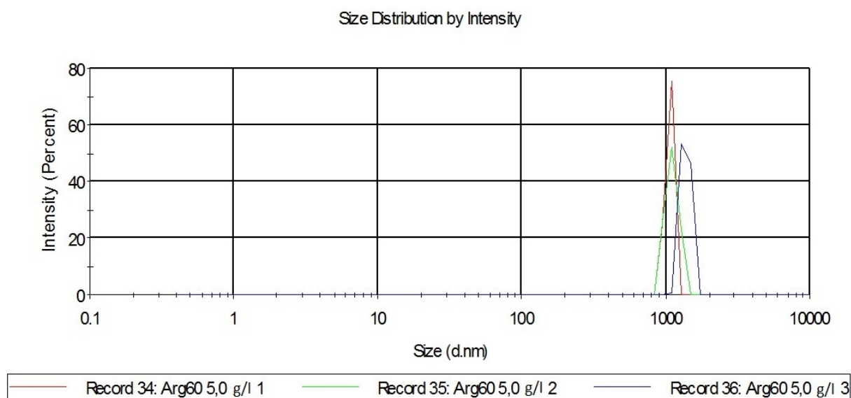
FIG. 1. The linear dimension of the particles on the base of the adducts C_{60}(C_6H_{12}NaN_4O_2)_8H_8 in aqueous ( \delta ) solutions at C = 5 \text{ g/dm}^3 (different curves correspond to the different times of observation (signal integration))
