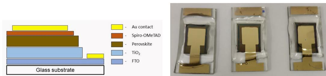
FIG. 2. Device architecture of the PSC (left) and the laboratory PSCs prepared in the Solar photovoltaic laboratory of IBCP RAS (right)
