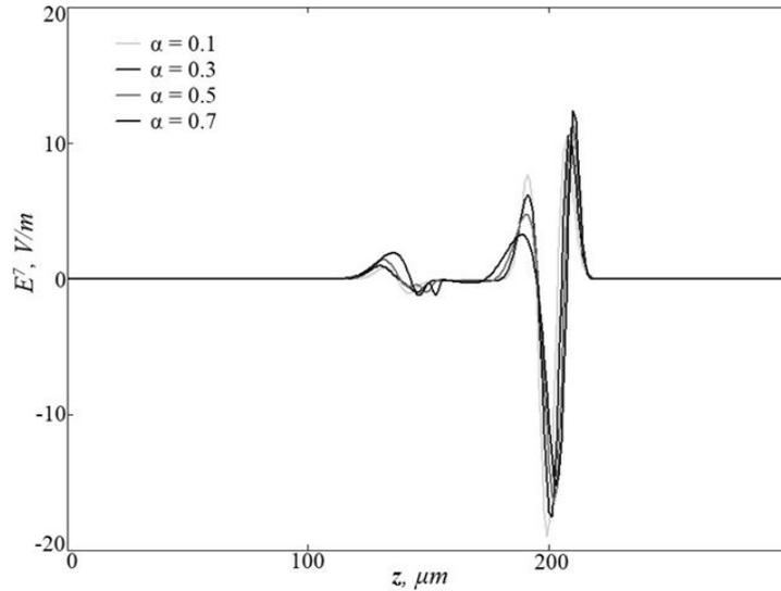
FIG. 3. Sections of a three-dimensional extremely short optical pulse in a photonic crystal made of CNTs with a superlattice, at a time instant of 4 ps, with different values of the modulation depth of the refractive index, at a fixed modulation period  $\chi = 2.5 \mu\text{m}$ :  $\alpha = 0.1, 0.3, 0.5, 0.7$
