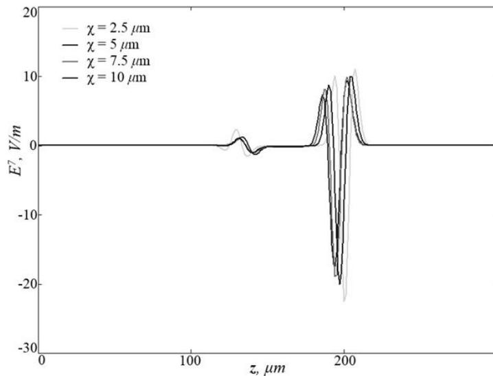
FIG. 4. The dynamics of propagation of a three-dimensional extremely short optical pulse in a photonic crystal of CNTs with a superlattice, at a time instant of 4 ps, with different values of the refractive index modulation period, at a fixed modulation depth  $\alpha = 0.3$ :  $\chi = 2.5 \mu\text{m}, 5 \mu\text{m}, 7.5 \mu\text{m}, 10 \mu\text{m}$
