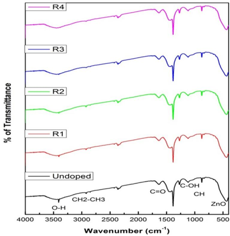
FIG. 2. FTIR spectrum of leaf extracted ZnO
