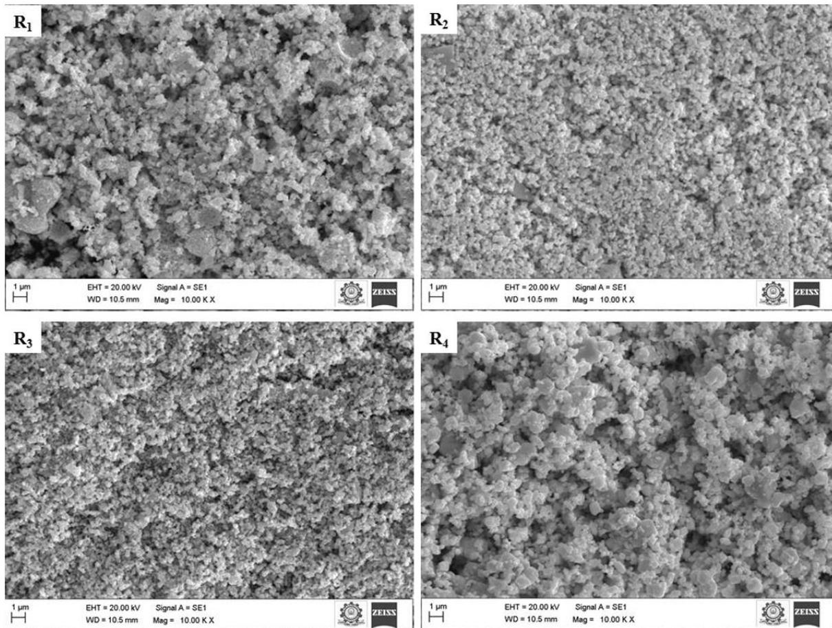
FIG. 3. The SEM image of prepared ZnO NPs
