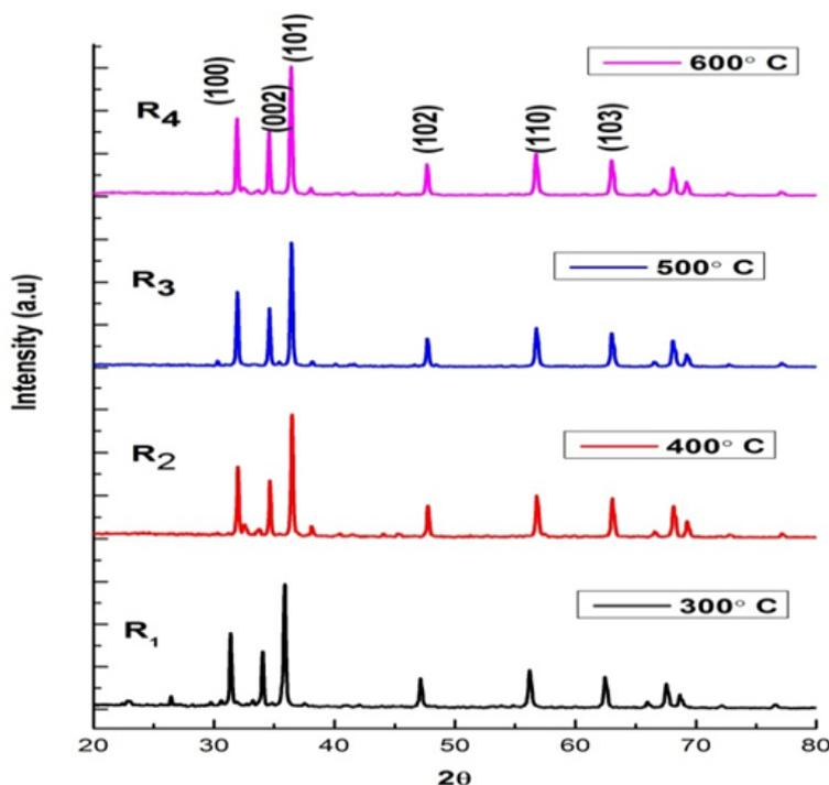
FIG. 1. XRD patterns of synthesized ZnO NPs
