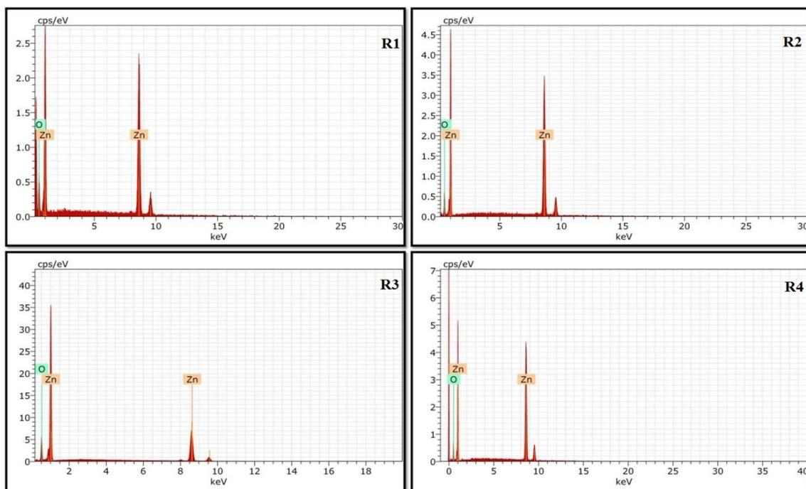
FIG. 4. The EDAX analysis of prepared ZnO NPs
