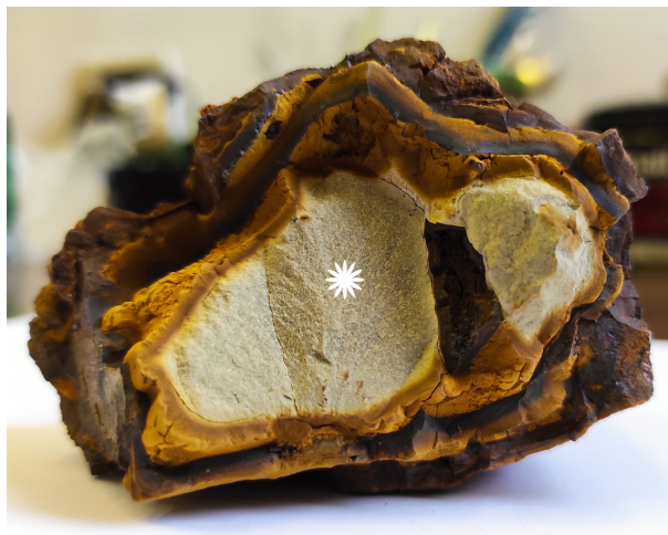
FIG. 1. General view of the sample: central zone – siderite (*), outer zones - cocentric aggregate of limonite (natural oxidation products)
