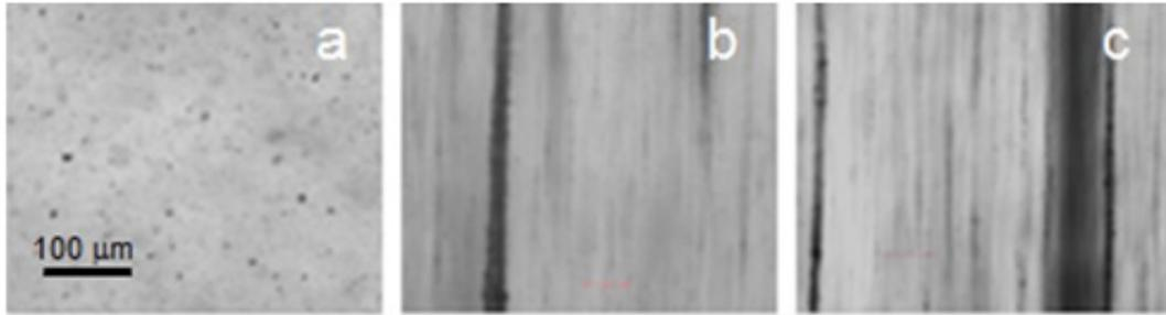
FIG. 2. Micrographs of a sample based on epoxy resin: a)  $H = 0$ ; b)  $H = 4$  kOe; c)  $H = 6$  kOe (the scale is the same for all images)
