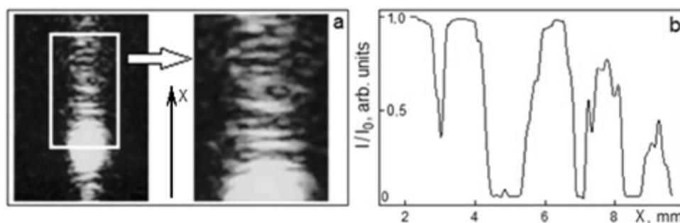
FIG. 4. Diffraction of laser radiation on selected agglomerate (sample based on epoxy resin,  $H = 4$  kOe): a) diffraction pattern at different scales; b) distribution of the relative intensity of diffracted light
