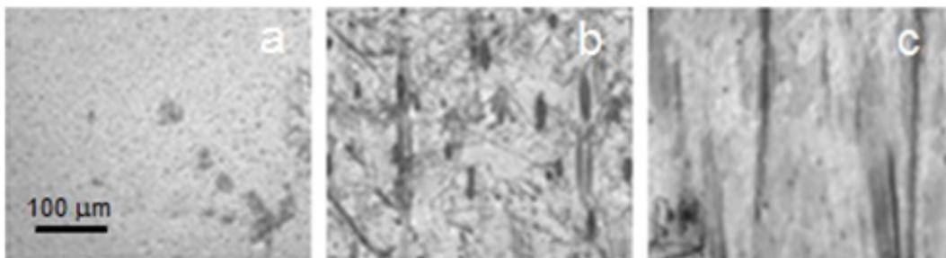
FIG. 1. Micrographs of a sample based on PVA at: a)  $H = 0$ ; b)  $H = 40$  Oe; c)  $H = 1000$  Oe (the scale is the same for all images)
