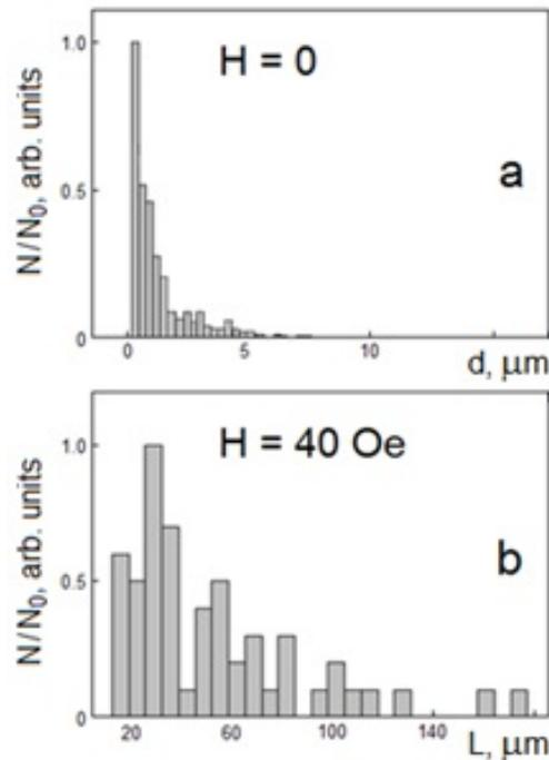
FIG. 3. Histograms of the distribution of the size of agglomerates in a sample with PVA: a) without field; b) in the field  $H = 40$  Oe
