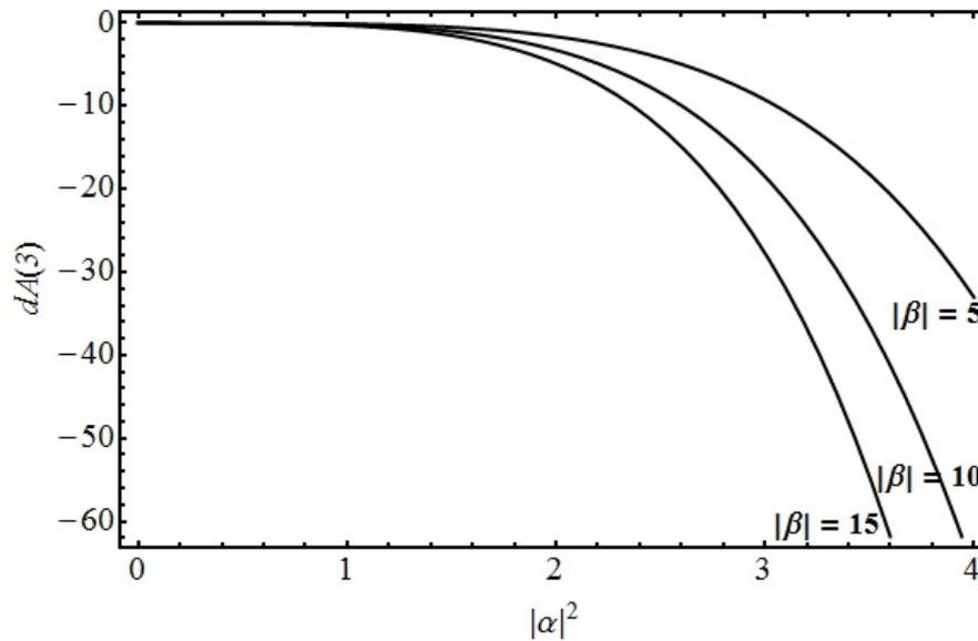
FIG. 5. Third-order photon antibunching  $d_A(3)$  with  $|\alpha|^2$  in the pump field up to first-order Hamiltonian interaction of sixth harmonic generation (when  $|\beta| = 5, 10, 15$  and  $|gt| = 10^{-5}$ )
