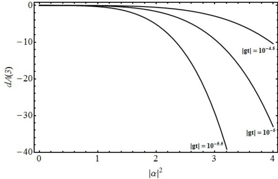
FIG. 7. Third-order photon antibunching  $d_A(3)$  with  $|\alpha|^2$  in the pump field up to first-order Hamiltonian interaction of sixth harmonic generation (when  $|\beta| = 5$  (arbitrarily value) and  $|gt| = 10^{-4.5}, 10^{-5}, 10^{-5.5}$ )
