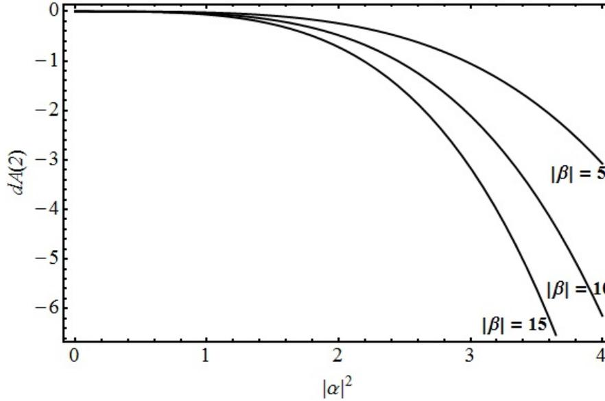
FIG. 4. Second-order photon antibunching  $d_A(2)$  with  $|\alpha|^2$  in the pump field up to first-order Hamiltonian interaction of sixth harmonic generation (when  $|\beta| = 5, 10, 15$  and  $|gt| = 10^{-5}$ )
