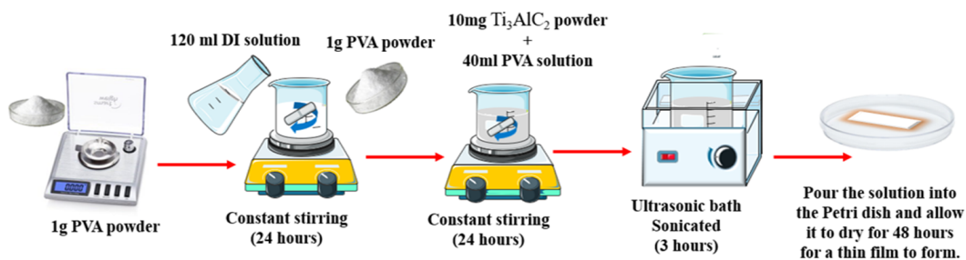
FIG. 1. Illustration of Ti_3AlC_2 PVA film preparation
