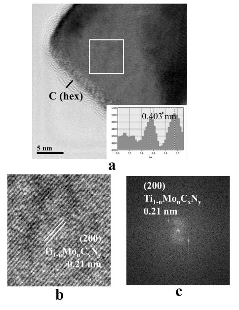
FIG. 5. Electron microscopic image (HRTEM) of (a) a nanocrystalline particle with a "core-shell" structure of the composition  $Ti_{1-n}Mo_nC_xN_y - Ni - Mo$  coated with carbon, enlarged image (b) and its fast Fourier transform results (c)
