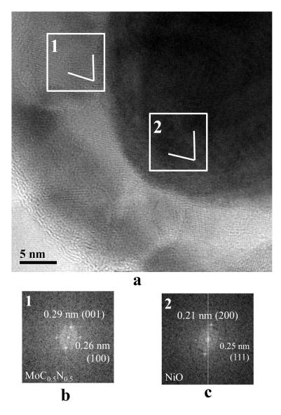
FIG. 3. Electron microscopic image of a nanocrystalline particle with a "core-shell" structure (a) of the  $Ti_{1-n}Mo_nC_xN_y - Ni - Mo$  tungsten-free hard alloy charge, taking into account the fast Fourier transform processing of various image sections containing  $MoC_{0.5}N_{0.5}$  (section 1) (b) and NiO (section 2) (c)
