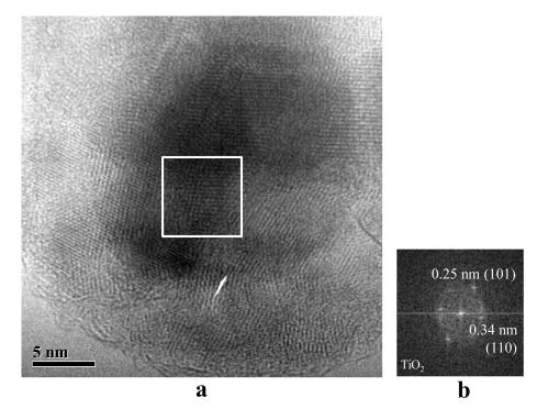
FIG. 4. Electron microscopic image of a nanocrystalline particle (a) of the  $Ti_{1-n}Mo_nC_xN_y - Ni - Mo$  alloy charge and FFT transformation of a section of the particle (b)
