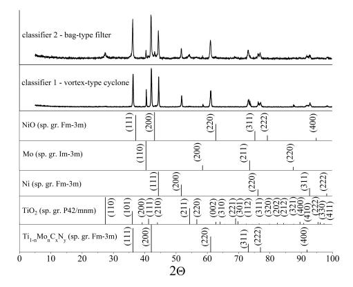
FIG. 1. Results of X-ray phase analysis of highly dispersed powders with a "core-shell" structure of the tungsten-free hard alloy charge based on titanium-molybdenum carbonitride  $Ti_{1-n}Mo_nC_xN_y$  with the participation of Ni and Mo formed during plasma-chemical synthesis in a low-temperature nitrogen plasma
