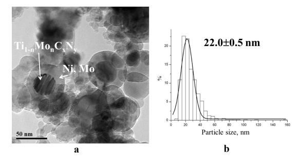
FIG. 2. HRTEM (a) of the nanocrystalline fraction of the processed mechanical mixture  $TiC_{0.5}N_{0.5}$  – Mo – Ni from classifier 2 – bag-type filter and particle size distribution histogram (b)
