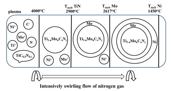
FIG. 7. Chemical mechanism of formation of nanocrystalline particles with a "core-shell" structure of the  $Ti_{1-n}Mo_nC_xN_y$ -Ni-Mo hard alloy charge, obtained by plasma-chemical synthesis in a low-temperature nitrogen plasma
