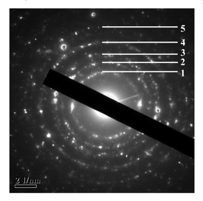
FIG. 6. Electron diffraction pattern of a polycrystalline sample of  $Ti_{1-n}Mo_nC_xN_y - Ni - Mo$
