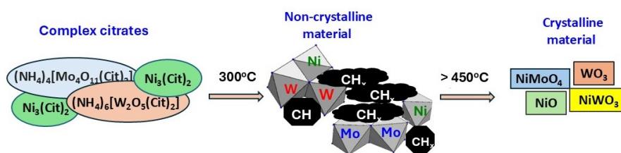
FIG. 5. Scheme on the possible reactions being occurred in the NiMoW precursor
