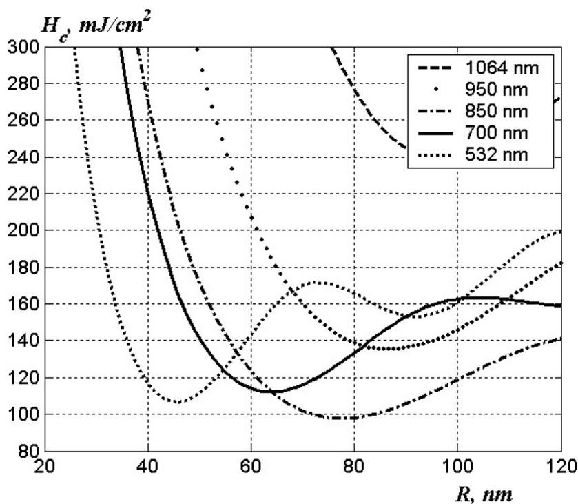
FIG. 3. Dependences of the critical energy density on the aluminum nanoparticle's radius in PETN matrix for the initiating wavelengths 532, 700, 850, 900 and 1064 nm
