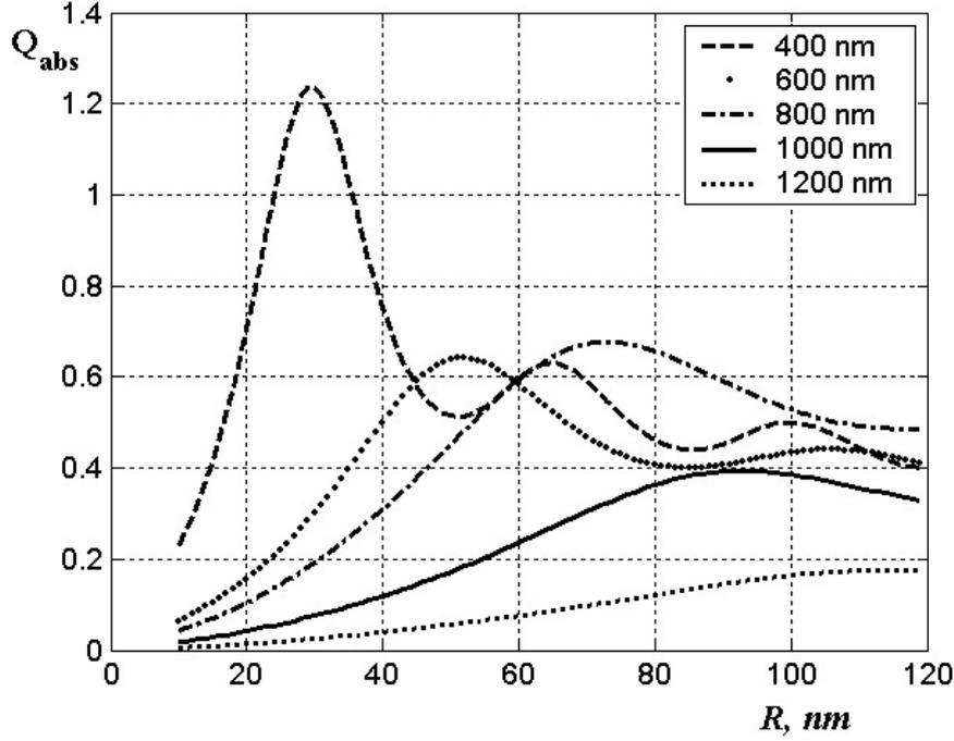
FIG. 1. Calculated dependences of the aluminium nanoparticles' absorptivity ( $Q_{abs}$ ) in PETN-matrix on the particles' sizes for wavelengths 400, 600, 800, 1000, 1200 nm
