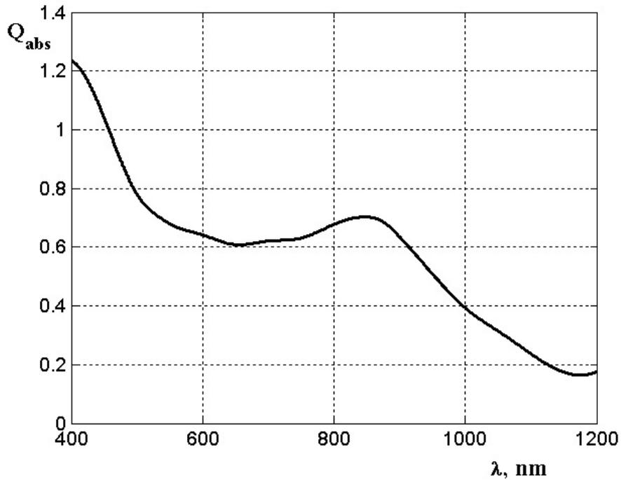
FIG. 2. Dependences of the aluminum nanoparticles' maximal absorptivity in PETN matrix on the initiating wavelength in a spectral range 400 – 1200 nm
