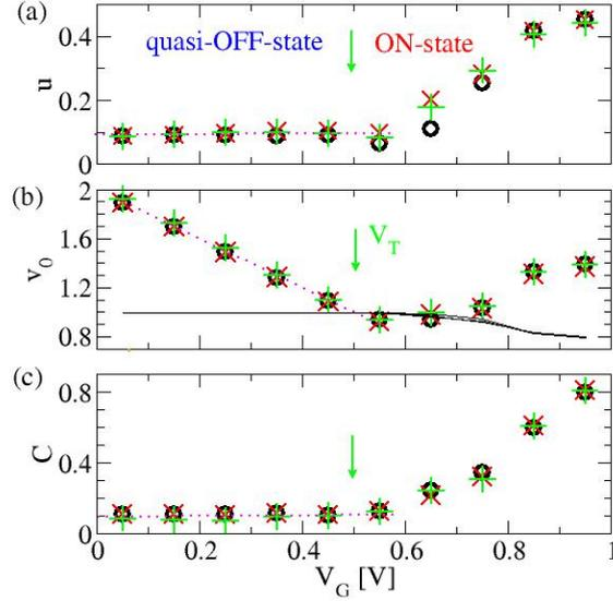
FIG. 3. Calibration functions (a)  $u(V_G)$ , (b)  $v_0(V_G)$ , and (c)  $C(V_G)$ , filled circles  $L = 22$  nm, symbols 'x'  $L = 26$  nm, and open rectangles  $L = 30$  nm. In dotted lines the four-constants-fit  $u = 0.09$ ,  $C = 0.1$ ,  $\beta = 2/V$ , and  $v_s^0 = -1V$ . The solid black line in (b) marks the position of  $m$ .
