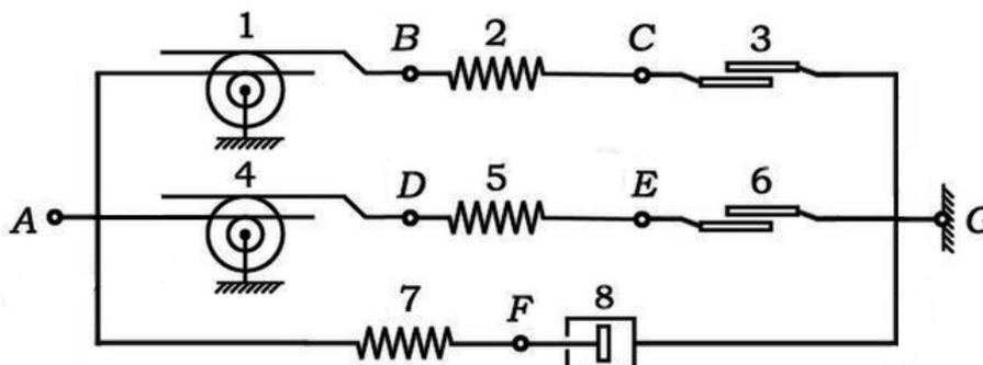
Fig. 1. Schematic of the model of the mechanical behavior of rubber
