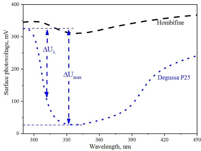
FIG. 3. SPV spectra of Degussa P25 and Hombifine powders
