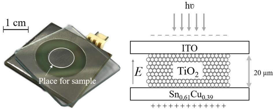
FIG. 1. Image and scheme of a cell for measuring SPV
