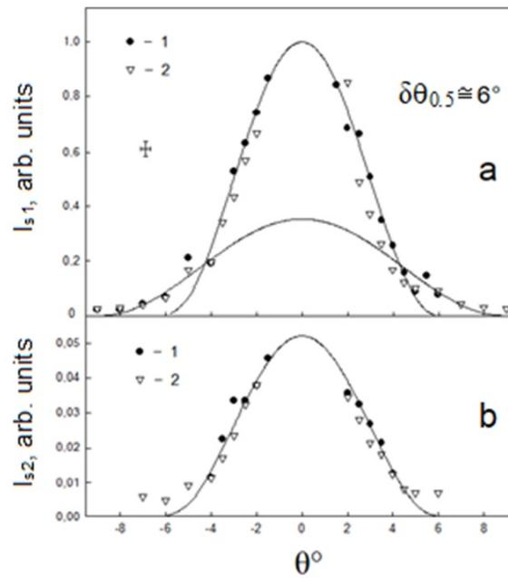
FIG. 1. Indicatrices of epoxy-based sample for registration of scattered light with polarization parallel (a) and orthogonal (b) to polarization  $p$  of incident beam. 1 – Perpendicular orientation of  $H$  to  $p$ , 2 – parallel orientation of  $H$  to  $p$
