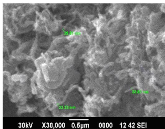
FIG. 1. SEM of CNT synthesized from Castor oil
