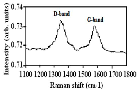
FIG. 3. Raman spectra of CNT synthesized from Castor oil
