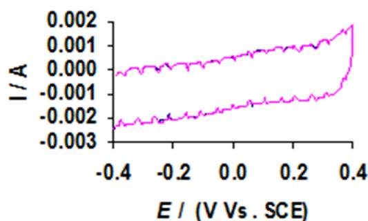
FIG. 4. CV of CNT in 30 % KOH; weight of electroactive material – 5 mg
