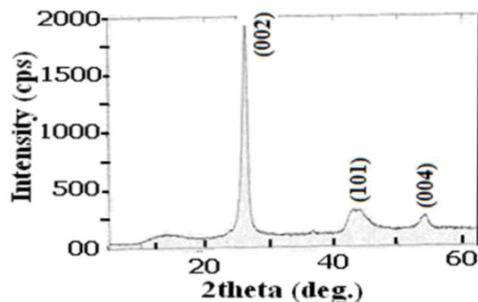
FIG. 2. XRD of CNT synthesized from Castor oil
