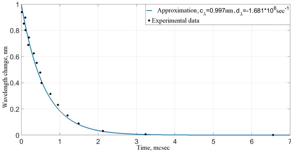
FIG. 2. Graph of VCSEL wavelength change during the cooling process
