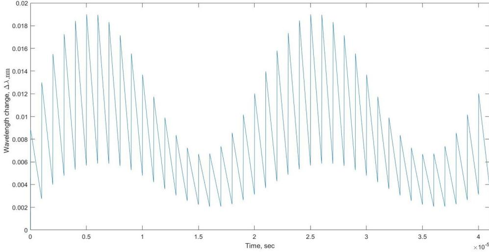
FIG. 3. VCSEL wavelength change with modulation amperage pulses
