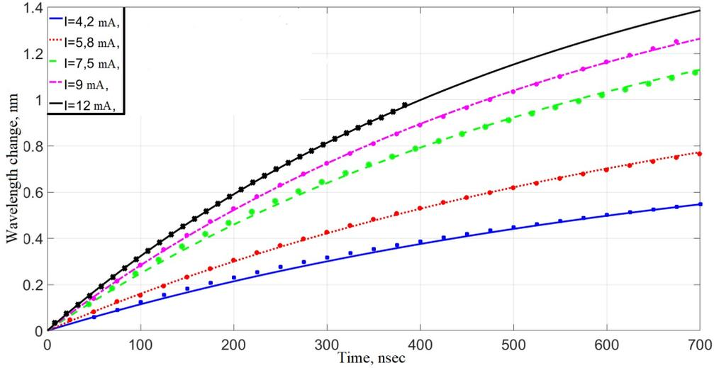
FIG. 1. VCSEL wavelength changes for different modulation amperages
