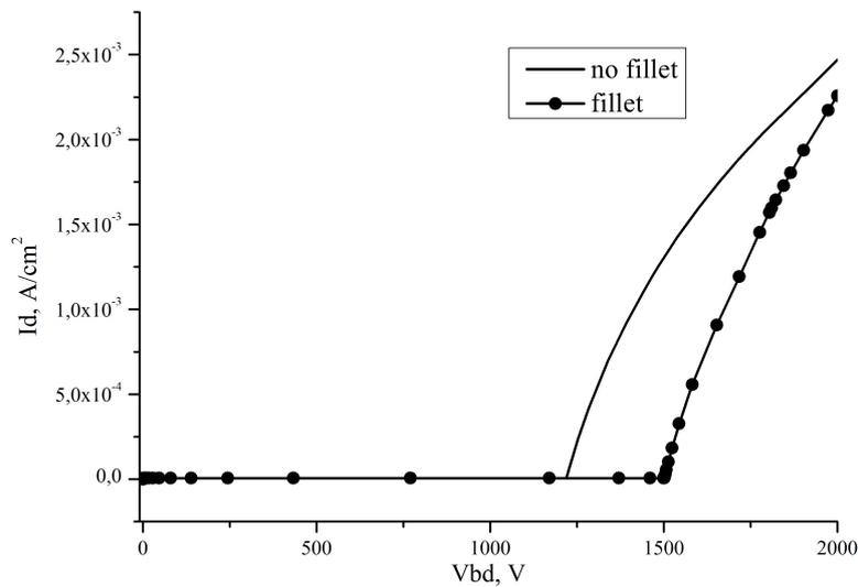
FIG. 3. Influence of drain p-region describing on SiC MOSFET breakdown voltage
