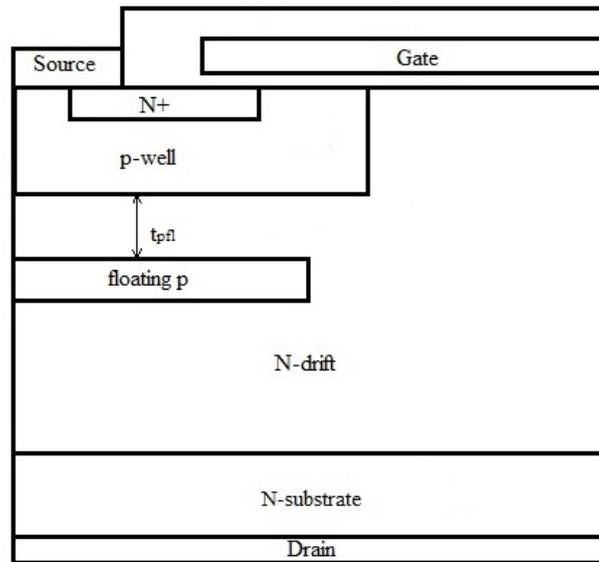
FIG. 10. Schematic image of SiC MOSFET with additional p-region in the drift region to increase the breakdown voltage
