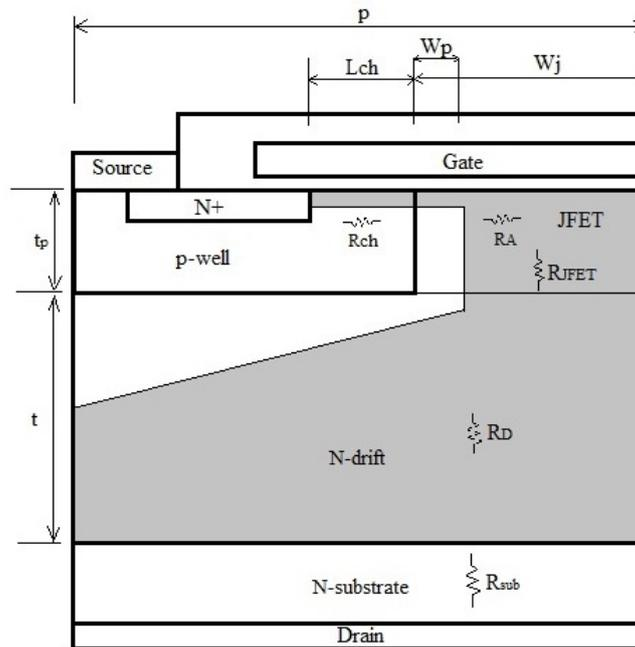
FIG. 1. Schematic image of SiC MOSFET,  $t_p$  – width of p-region,  $t$  – drift region width,  $p$  – half length of the structure,  $L_{ch}$  – channel length,  $W_p$  – width of p-n junction p-base/N-JFET,  $W_j$  – JFET region width
