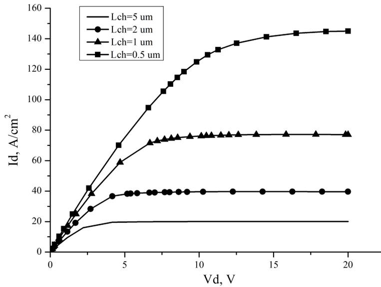
FIG. 4. Influence of length channel Lch on the transistor current-voltage characteristics at 15 V gate voltage
