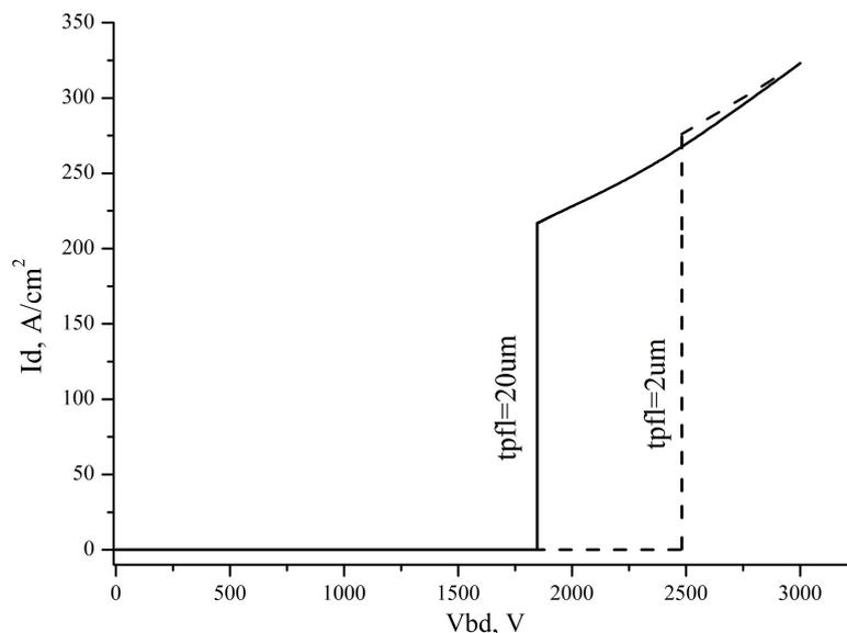
FIG. 11. Breakdown voltage of SiC MOSFET with additional p-region in drift region with different distances from p-base to additional p-region  $tp_{fl}$
