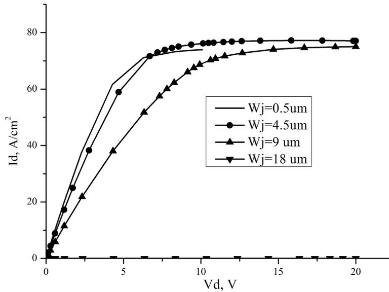
FIG. 6. Influence of JFET region width  $W_j$  on current-voltage characteristics at 15V gate voltage
