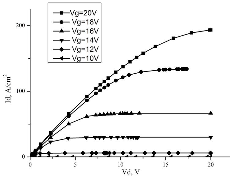
FIG. 7. Current-voltage characteristics of the SiC MOSFET
