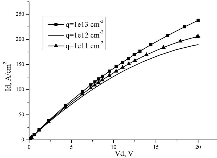
FIG. 2. The influence of positive charge density  $q$  at  $\text{SiO}_2/\text{SiC}$  heterojunction on MOSFET current-voltage characteristics at 20 V gate voltage
