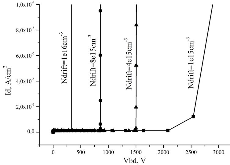
FIG. 8. Dependence of SiC MOSFET breakdown voltage on drift region doping concentration  $N_{drift}$
