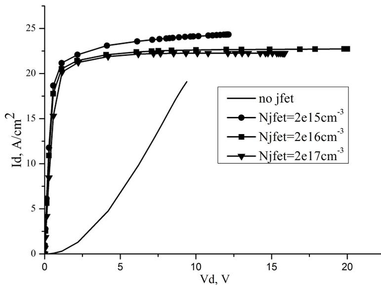
FIG. 5. Dependence of current-voltage characteristics on doping concentration of JFET region Njfet at 15 V gate voltage
