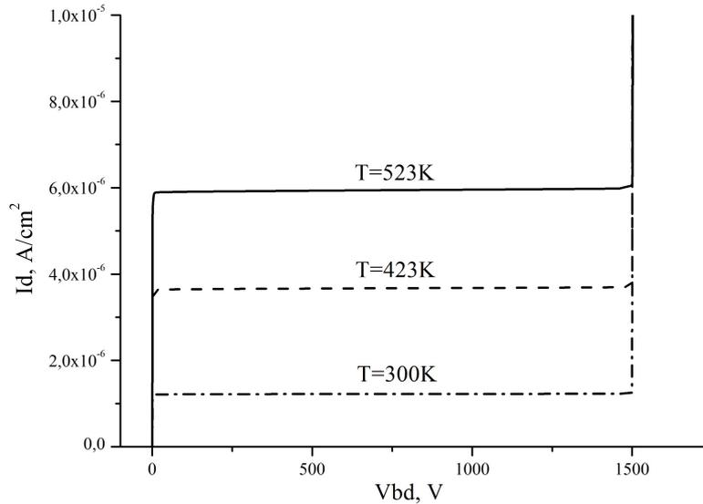
FIG. 9. SiC MOSFET breakdown voltage at different temperatures
