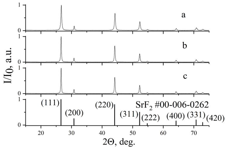
FIG. 1. XRD patterns of the samples # 1(a), 2(b), 3 (c) and  $\text{SrF}_2$
