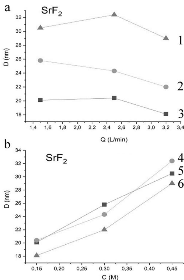
FIG. 3. The dependence of the coherent scattering values of  $D$  strontium fluoride nanoparticles synthesized in a reactor with swirling flows at different on the flow rates (a) and the concentration of strontium nitrate (b). Notations: M  $\text{Sr}(\text{NO}_3)_2$  is equal to 0.45 (1); 0.30 (2); 0.15 (3);  $Q$  is equal to 2.5 L/min (4); 1.5 L/min (5); and 3.2 L/min (6).
