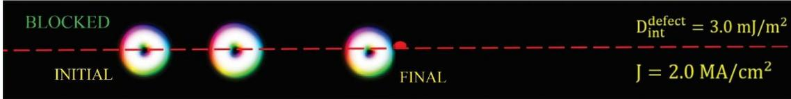
Fig. S19 Schematic representation of the passing state; the skyrmionium stops before colliding with the defect.
