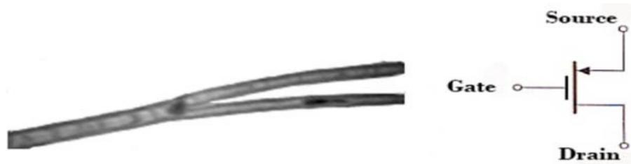
FIG. 3. SEM image (a) and schematic diagram (b) of a transistor built on a Y-shaped carbon nanotube
