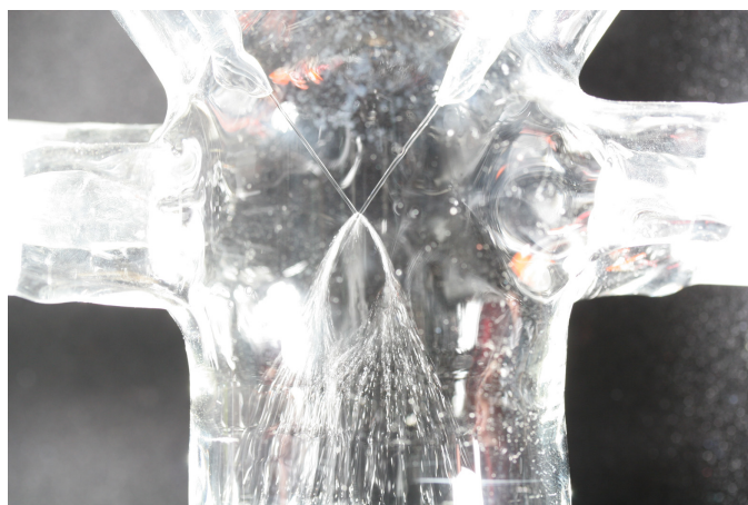
FIG. 1. Liquid sheet formation at the jets collision in the free impinging-jets microreactor
