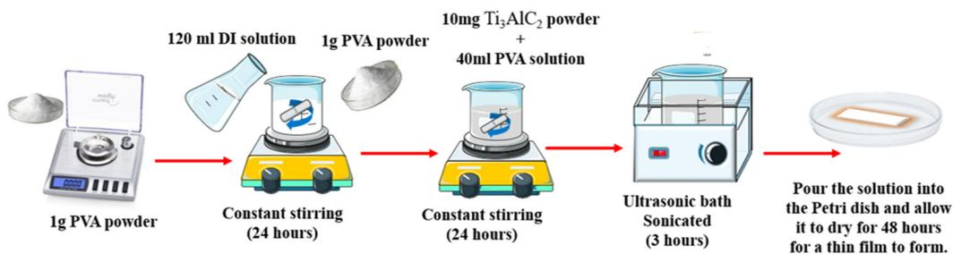
FIG. 1. Illustration of  $Ti_3AlC_2$  PVA film preparation
