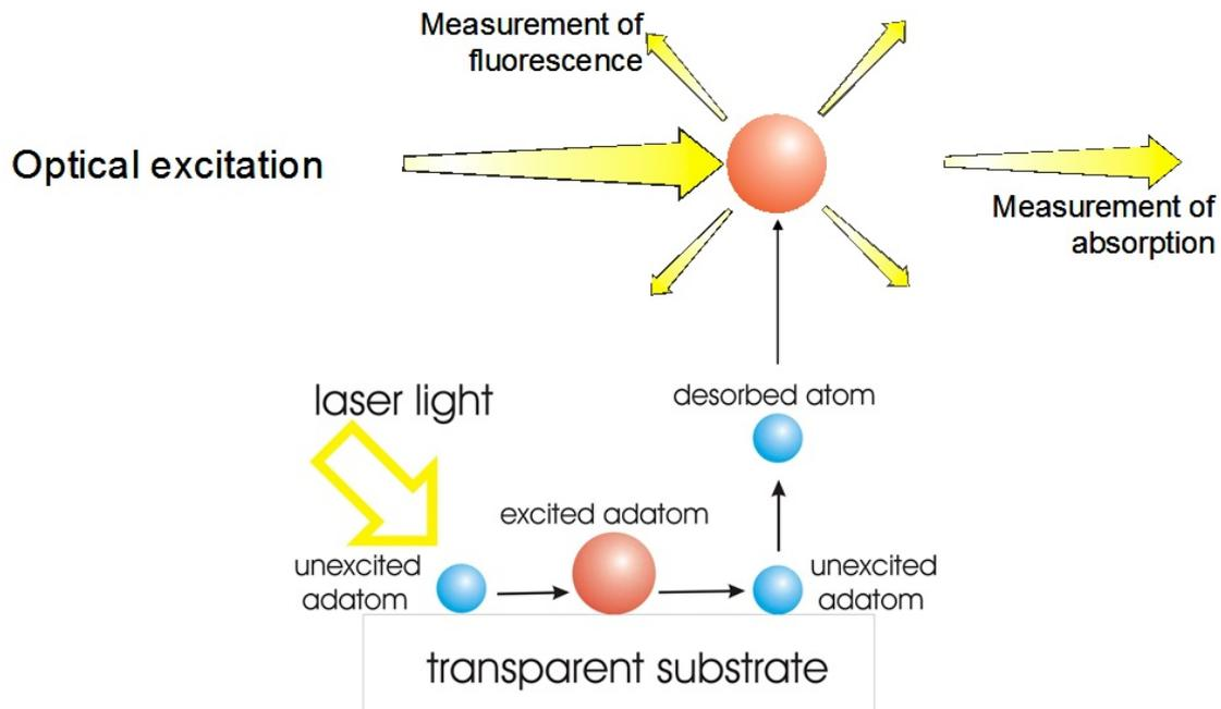
FIG. 3. Registration of photodesorption via absorption or fluorescence measurements
