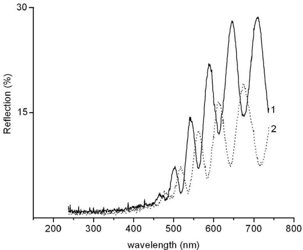
FIG. 4. Reflection spectra of the anodized 20 min films with electrochemically deposited silver nanoparticles in reference to Al mirror. The solid curve (1) is spectrum for the input angle of  $20^\circ$ . The dot curve (2) is spectrum for the input angle of  $40^\circ$ . It is seen that the high contrast interference reflection spectra are shifted one half of phase when changing the input angle from  $20^\circ$  to  $40^\circ$
