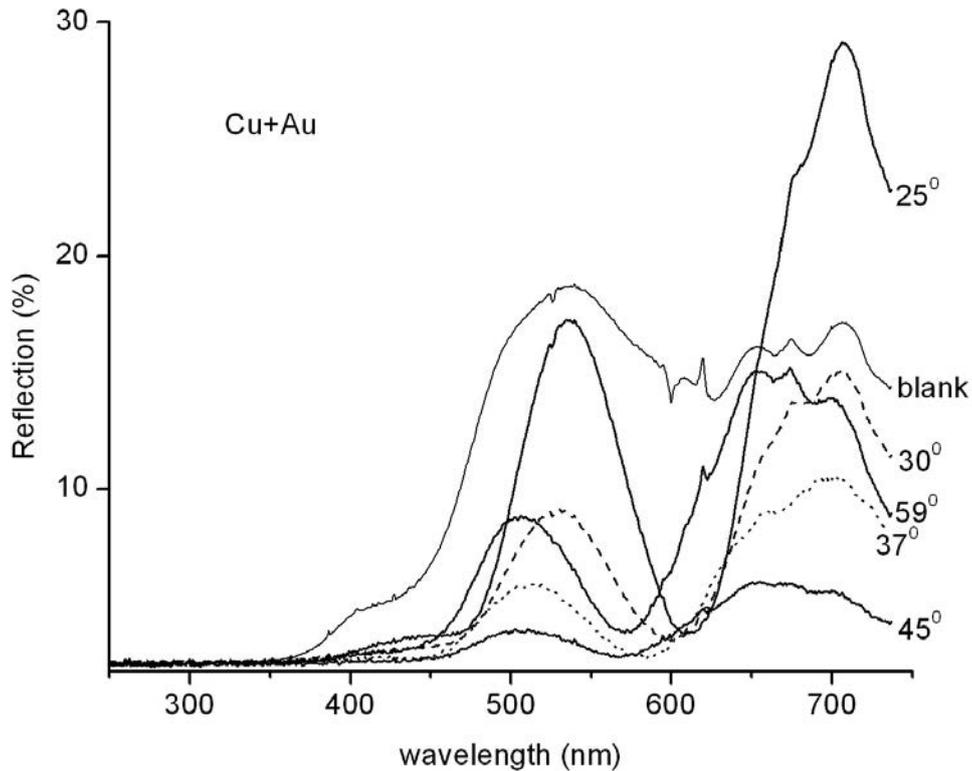
FIG. 3. The reflection spectra under different incident angles. The solid curve (blank) is reflection spectrum of the blank AAOF for the input angle of light  $25^\circ$
