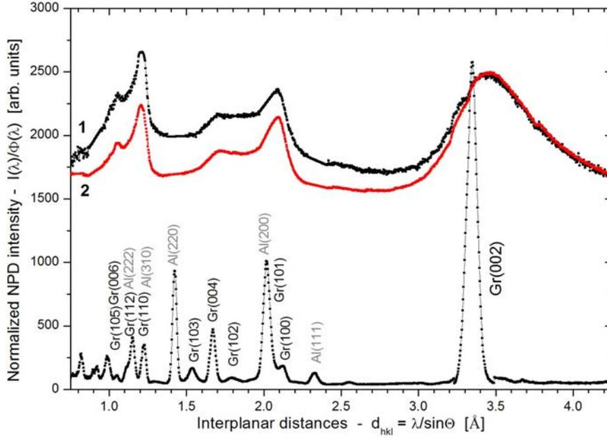
FIG. 2. NPD of shungites Sh1 (1) and Sh2 (2) recorded at  $T=20$  K after extraction of Al(hkl) reflections. Scattering angle  $2\Theta = 44.7^\circ$ . The data are normalized per neutron flux intensity  $\Phi(\lambda)$  at each neutron wave length  $\lambda$ ; Gr(hkl) (black) and Al(hkl) (gray) denote characteristic diffraction peaks of spectral graphite and cryostat (alongside with sample holder) aluminum at different Miller indexes, respectively
