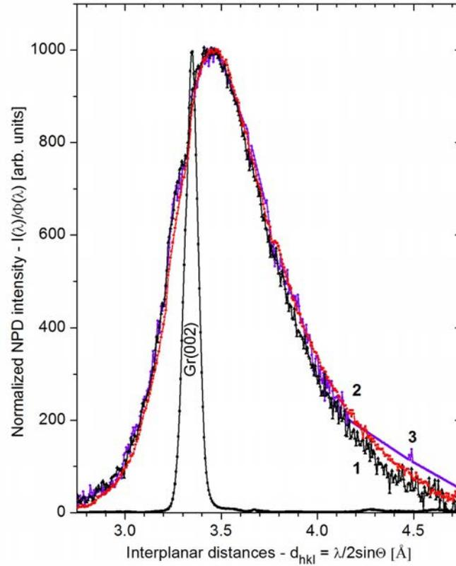
FIG. 3. NDP fragments of spectral graphite (Gr) and shungites Sh1 (1), Sh2 (2), and Sh3 (3) in the region of Gr(002) diffraction peaks;  $T=20$  K; scattering angle  $2\Theta = 44.7^\circ$ . The data are normalized per neutron flux intensity  $\Phi(\lambda)$  at each wave length of incident neutrons  $\lambda$ ; after a linear background subtraction, the intensity maxima of all the peaks are normalized to 1000 arbitrary units
