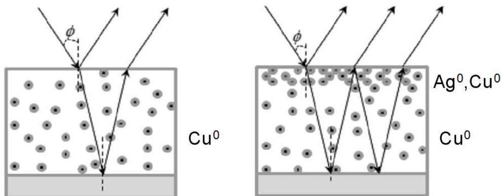
FIG. 5. Scheme of formation of the interference color
