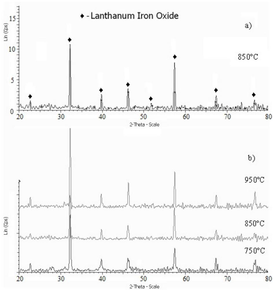
FIG. 4. XRD pattern of  $\text{La}_{0.9}\text{Sr}_{0.1}\text{FeO}_3$  sample heated at  $850^\circ\text{C}$  (a) and stack XRD diagram of  $\text{La}_{0.9}\text{Sr}_{0.1}\text{FeO}_3$  heated at  $750^\circ\text{C}$ ,  $850^\circ\text{C}$  and  $950^\circ\text{C}$  (b) ( $t=1$  h)
