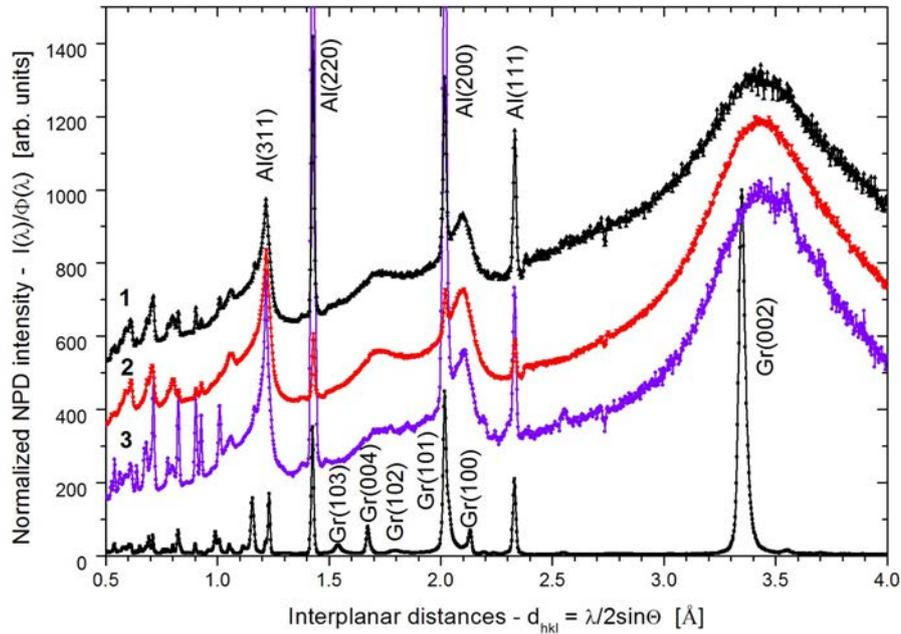
FIG. 1. NPD of spectral graphite (Gr) and shungites Sh1 (1), Sh2 (2), and Sh3 (3) recorded at  $T=20$  K. Scattering angle  $2\Theta = 117.4^\circ$ . The data are normalized per neutron flux intensity  $\Phi(\lambda)$  at each neutron wave length  $\lambda$ ; Gr(hkl) and Al(hkl) denote characteristic diffraction peaks of spectral graphite and cryostat aluminum at different Miller indexes, respectively
