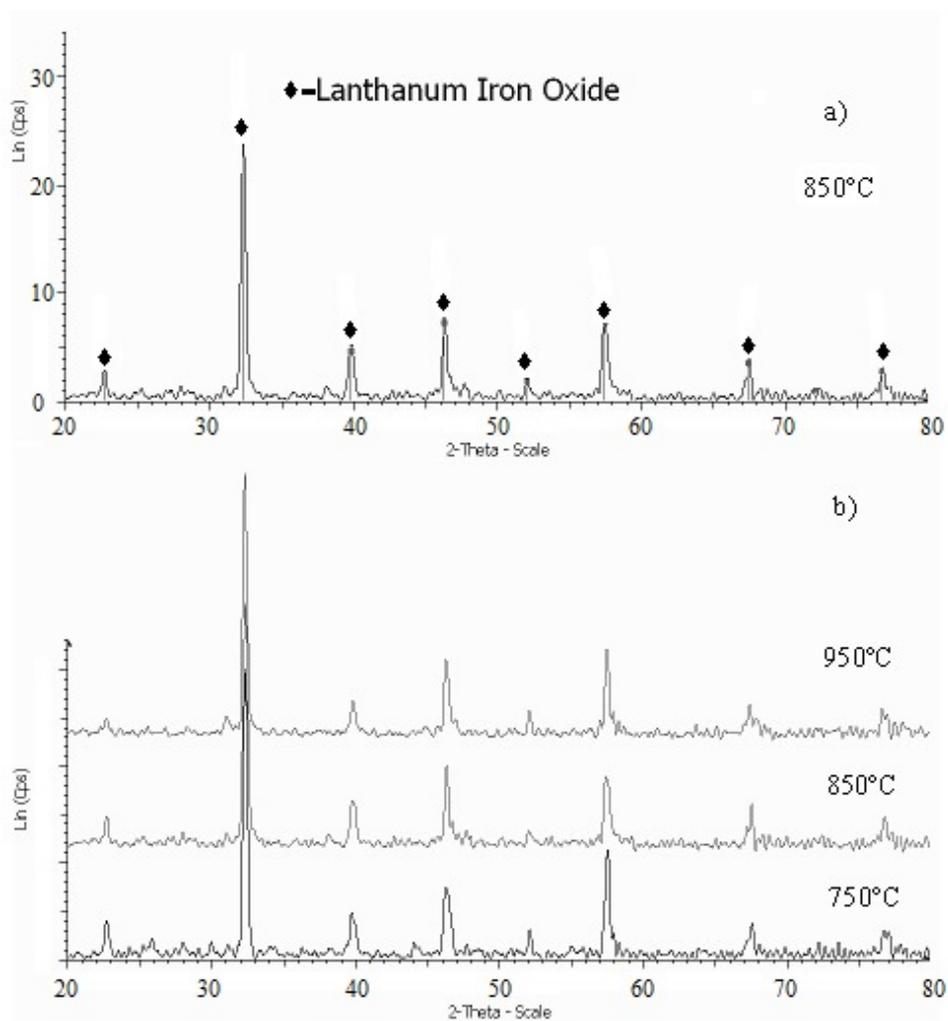
FIG. 6. XRD pattern of  $\text{La}_{0.7}\text{Sr}_{0.3}\text{FeO}_3$  sample heated at 850°C (a) and stack XRD diagram of  $\text{La}_{0.7}\text{Sr}_{0.3}\text{FeO}_3$  heated 750°C, 850°C and 950°C (b) ( $t=1$  h)
