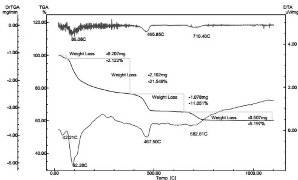
FIG. 1. TGA/DTA diagram of powder sample
