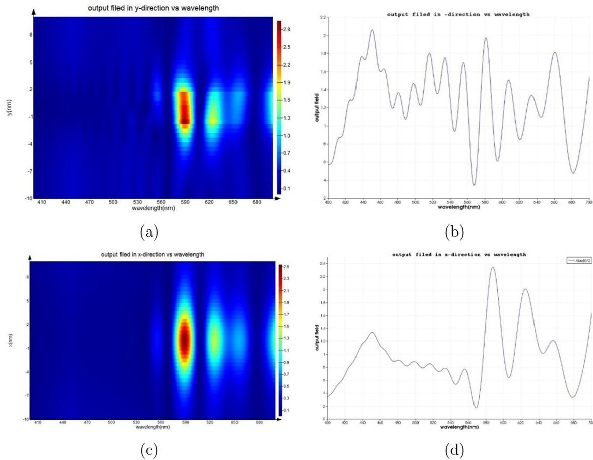
FIG. 4. Results with 250 nm period grating: (a) the distribution intensity with  $y$  on the line of  $x=0, z=0$  (b) the curve of enhancement of  $y$  component of electric field in  $y=0$  versus wavelength (c) the intensity distribution intensity with an  $x$  on the line of  $y=0, z=0$  (d) the curve of enhancement of the  $x$  component of electric field in  $x=0$  versus wavelength
