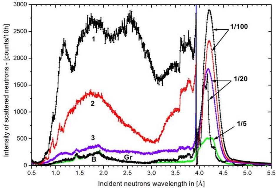
FIG. 4. Time-of-flight INS spectra from shungites Sh1 (1=100g), Sh2 (2=96g), Sh3 (3=10g) and spectral graphite (Gr=10g). Curve B presents background from Al cryostat and sample holder material.  $T=20\text{K}$ . The intensity of elastic peaks is 100-fold, 20-fold, and 5-fold reduced for Sh1 and Sh2, Sh3 and graphite, and background, respectively. Spectra are normalized per 10 hours exposition time at constant power of the IBR-2 equal 1.9 MW
