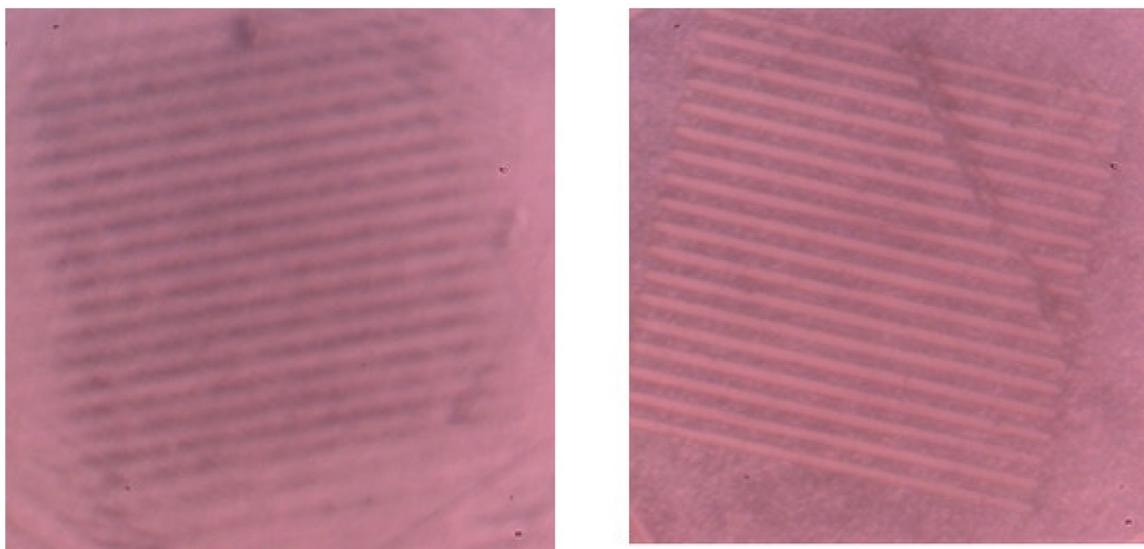
FIG. 5. (a) microscopic image of the sodium deposits on sapphire substrate obtained via physical vapor deposition under simultaneous laser illumination through the mire with  $10\ \mu\text{m}$  periodicity shown in (b)
