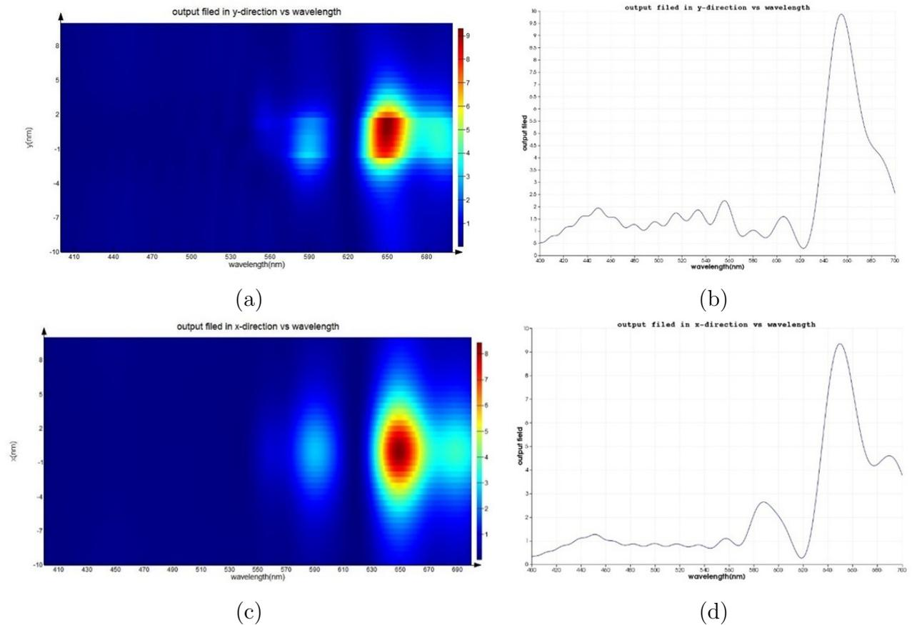
FIG. 5. Results with 300 nm period of the grating: (a) the distribution intensity with  $y$  on the line of  $x=0$ ,  $z=0$  (b) the curve of enhancement of  $y$  component of electric field in  $y=0$  versus wavelength (c) the intensity distribution intensity with an  $x$  on the line of  $y=0$ ,  $z=0$  (d) the curve of enhancement of the  $x$  component of electric field in  $x=0$  versus wavelength
