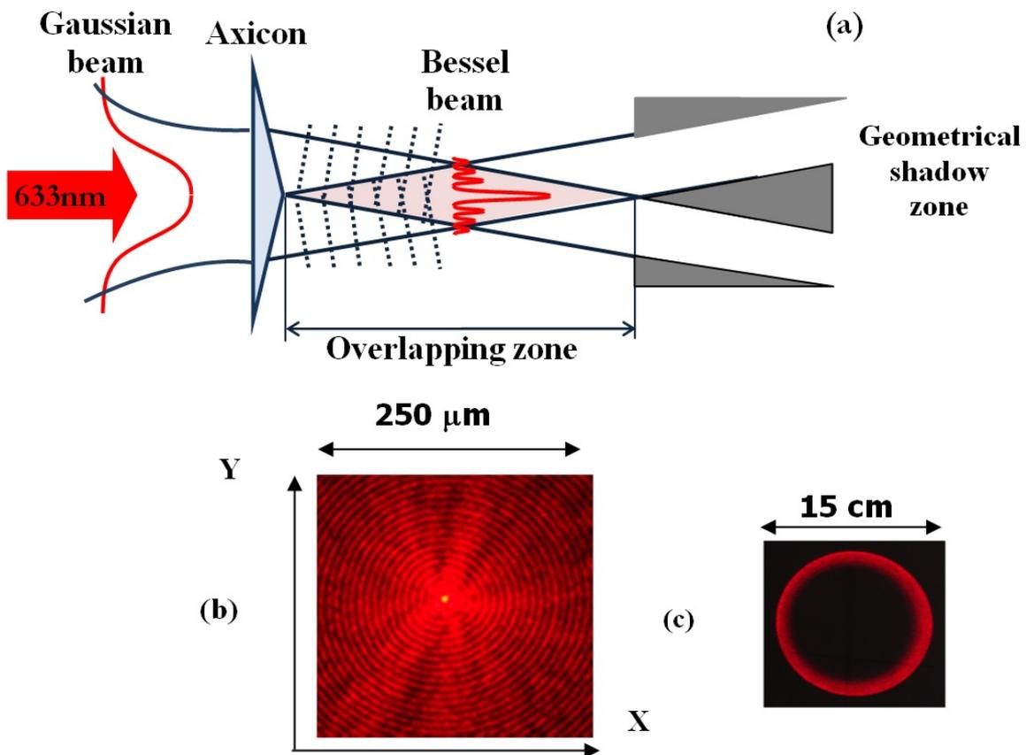
FIG. 6. (a) Experimental scheme illustrating the formation of Bessel beam by an axicon. (b) Fragment of transverse intensity distribution of Bessel beam formed by an axicon with aperture cone angle  $175^\circ$  in the overlapping zone of the beams. The number of rings reaches up to 500. (c) Ring pattern at the distance of 2 m behind the overlapping zone, where the beams become divergent
