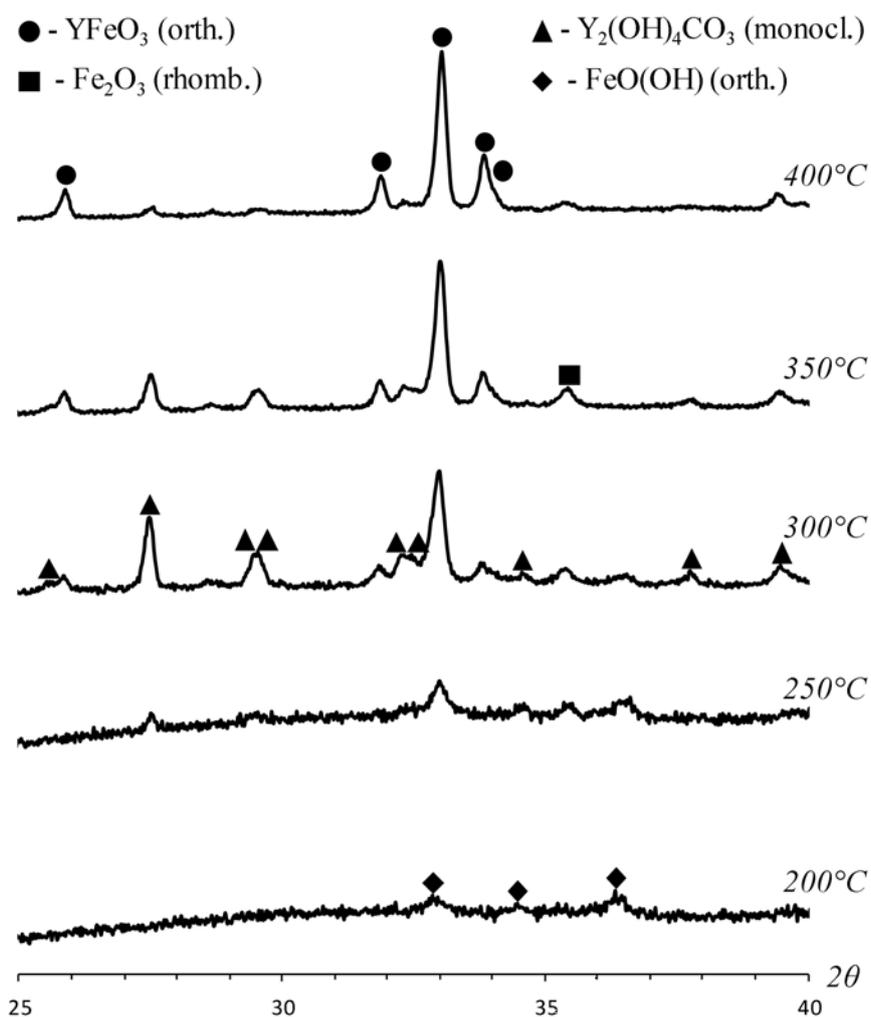
FIG. 1. X-ray diffractograms of the hydrothermal synthesis products
