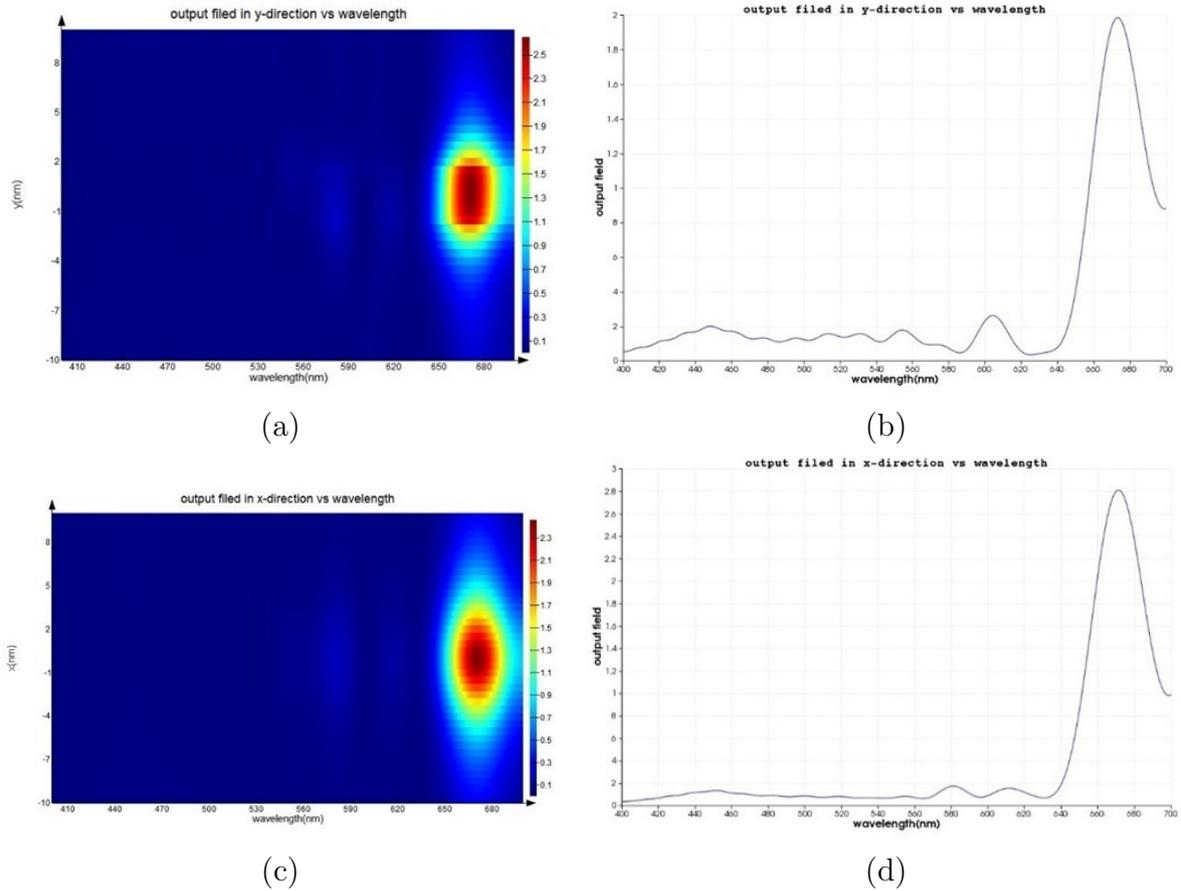
FIG. 3. Results with 200 nm period grating: (a) the distribution intensity with  $y$  on the line of  $x=0, z=0$  (b) the curve of enhancement of  $y$  component of electric field in  $y=0$  versus wavelength (c) the intensity distribution intensity with an  $x$  on the line of  $y=0, z=0$  (d) the curve of enhancement of the  $x$  component of electric field in  $x=0$  versus wavelength
