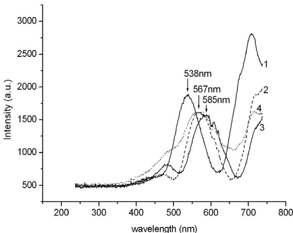
FIG. 8. Reflection spectra of Cu–Ag metalized AAOF (1) with water (2), ethanol (3) and dimethylsulfoxide (4)
