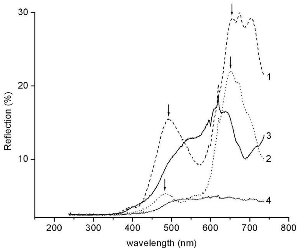
FIG. 2. Reflection spectra of the anodized films with chemical deposited gold (1) and silver (2) nanoparticles by substitution of copper in reference to Al mirror. The solid curve (3) is spectrum of the anodized film with Cu. The solid curve (4) is spectrum of the blank anodized film. It is seen that the difference between the maximum and minimum increases. The input angle of light is  $75^\circ$
