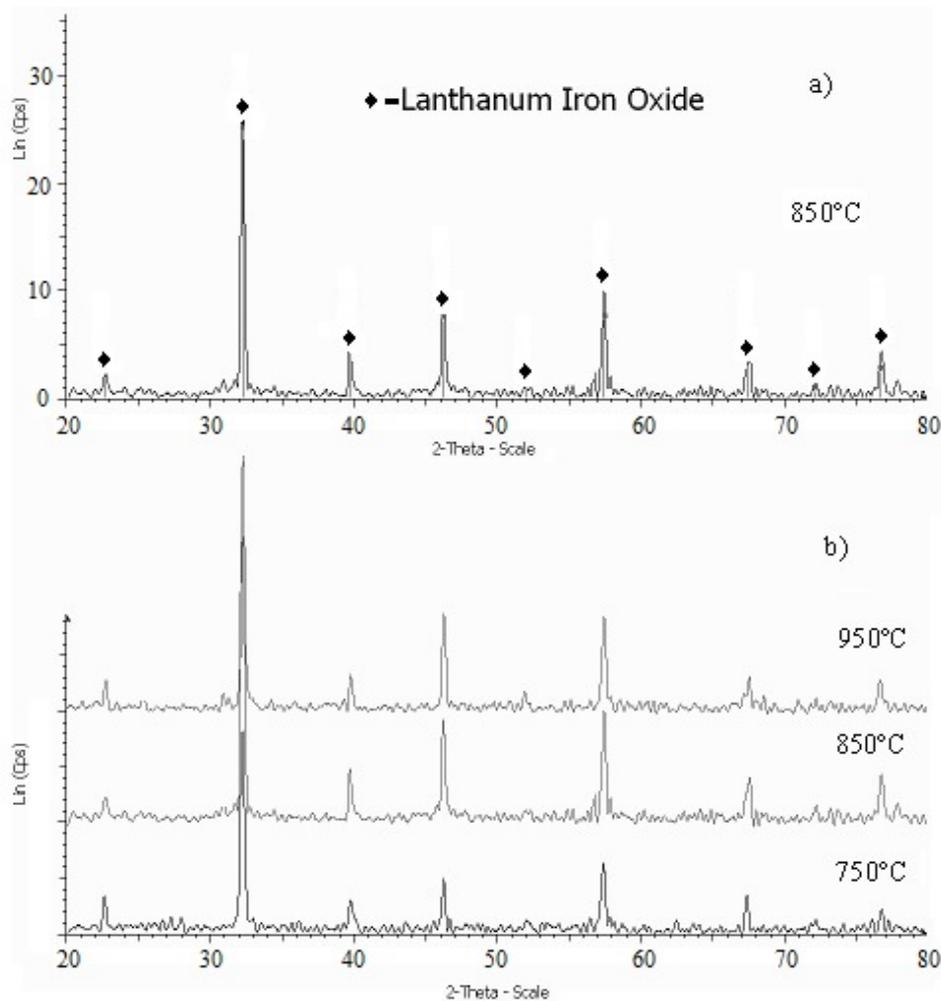
FIG. 5. XRD pattern of  $\text{La}_{0.8}\text{Sr}_{0.2}\text{FeO}_3$  sample heated at  $850^\circ\text{C}$  (a) stack XRD diagram of  $\text{La}_{0.8}\text{Sr}_{0.2}\text{FeO}_3$  heated at  $750^\circ\text{C}$ ,  $850^\circ\text{C}$  and  $950^\circ\text{C}$  (b) ( $t=1$  h)
