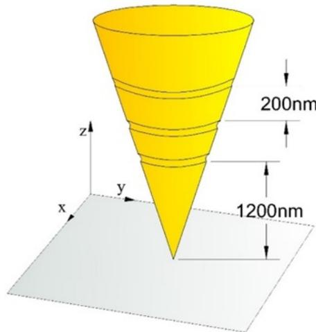
FIG. 1. Considered shape for optical antenna
