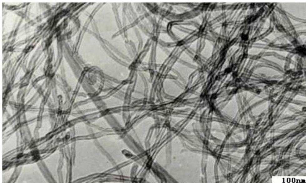
FIG. 1. Typical electronic photo of carbon multiwall nanotubes, produced by Bayer corporation (Germany) ( $\times 10^5$ )
