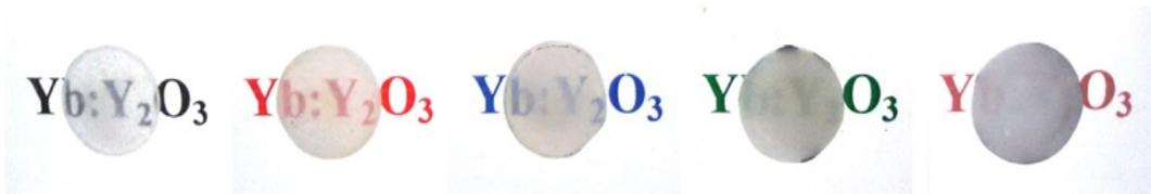
FIG. 3. Photograph of sintered pellets of Yb(1 mol%):  $Y_2O_3$  prepared using different surfactant concentrations: (a) 5 wt%, (b) 10 wt%, (c) 15 wt%, (d) 20 wt% and (e) 30 wt%
