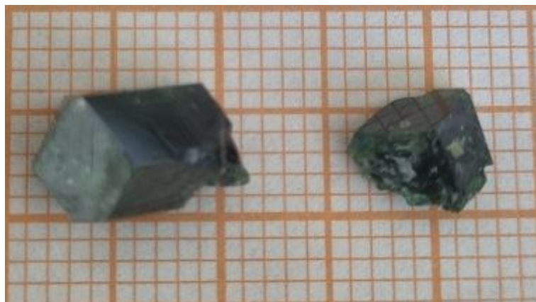
FIG. 2. External view of \text{HoFe}_3(\text{BO}_3)_4 single crystals grown by the flux method from a bismuth borate-based melt
